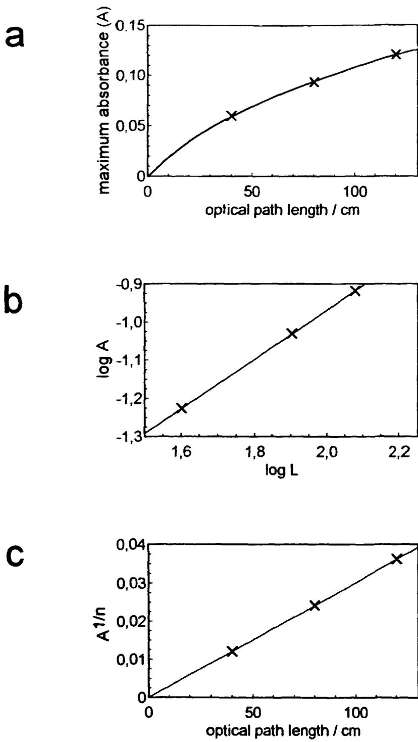
**FIGURE 1.** Measurements of the relation between optical path length,  $L$ , and OH radical absorbance monitored by the radical UV absorption at 309 nm by pulse radiolysis of 10 mbar  $H_2O$  and 990 mbar  $SF_6$ . The optical band pass is 1.2 Å. The absorbance is calculated as  $\log(I_0/I)$ . The slope in Figure b is 0.637 which also is the  $n$ -factor.
