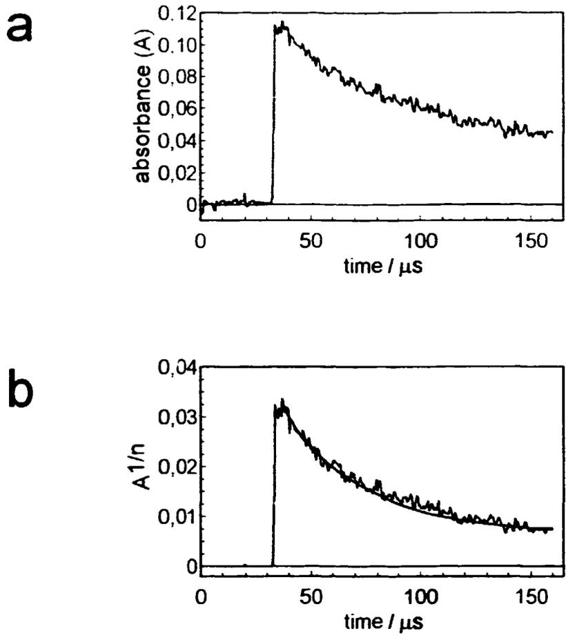
**FIGURE 2.** Figure a shows an OH transient without correction. The same corrected transient is shown in Figure b using an n-value of 0.637. The solid line is that predicted by modelling. The OH radicals were generated by pulse radiolysis of 10 mbar H<sub>2</sub>O and 990 mbar SF<sub>6</sub> and monitored by the UV absorption at 309 nm. The optical band pass is 1.2 Å and the path length is 120 cm. The absorbance is calculated as  $\log(I_0/I)$ .
