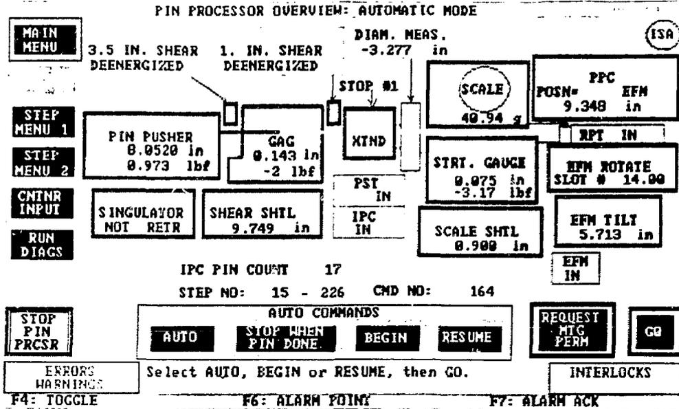
Figure 3 Pin Processor Operator Control Automatic Overview Screen
