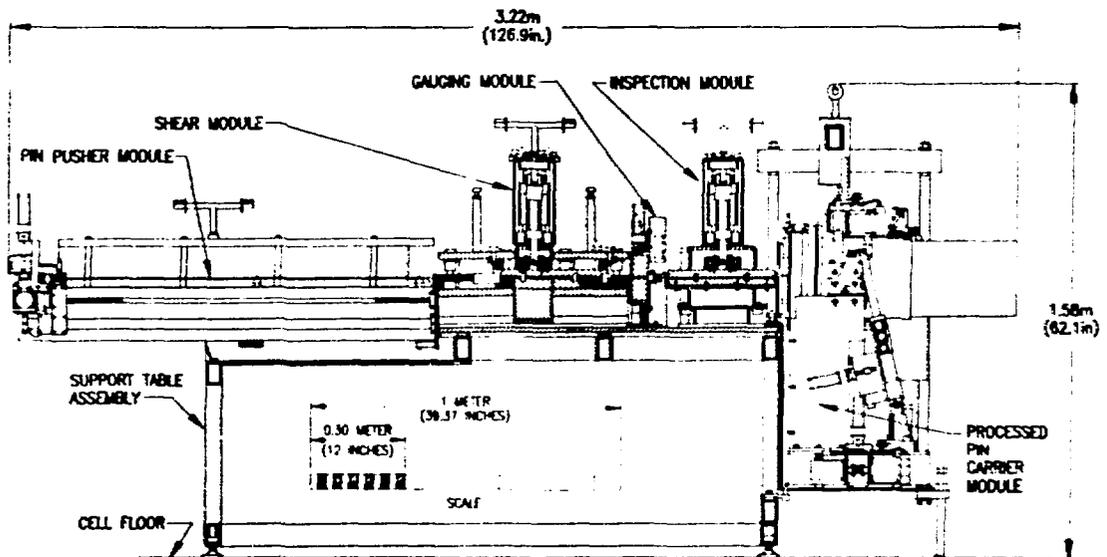
Figure 2 Pin Processor - Section Through Pin Path
