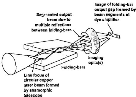
Fig. 2. A schematic representation of the mirror-pair, or folding-bar apparatus used to homogenize and reformat a circular copper laser pump beam into a generally rectangular shape at a dye amplifier for efficient overlap with the dye laser beam.
