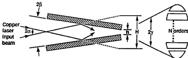
Fig. 3. A general schematic diagram of folding bars showing the divergence half-angle of the focused copper input beam,  $\alpha$ , the folding-bar wedge half-angle,  $\beta$ , the projected height of the copper beam in the plane of the output gap,  $H$ , the folding-bar output gap,  $h$ , the number of orders in the output,  $N$ , and the divergence half-angle of the output,  $\gamma$ .
