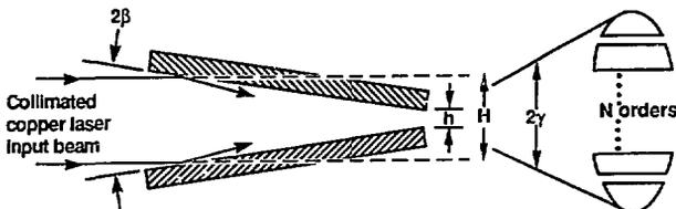
Fig. 4. A schematic diagram of folding bars similar to Fig. 3 but with a collimated copper laser input beam ( $\alpha = 0$ ).
