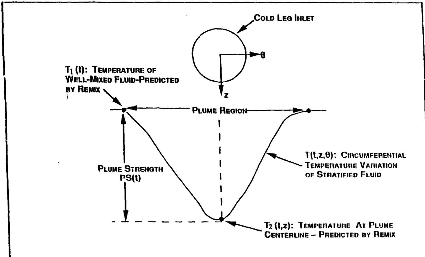
Fig. 3. Thermal streaming results in formation of plume, that is, a circumferential variation of fluid temperature on the inner surface of vessel.
