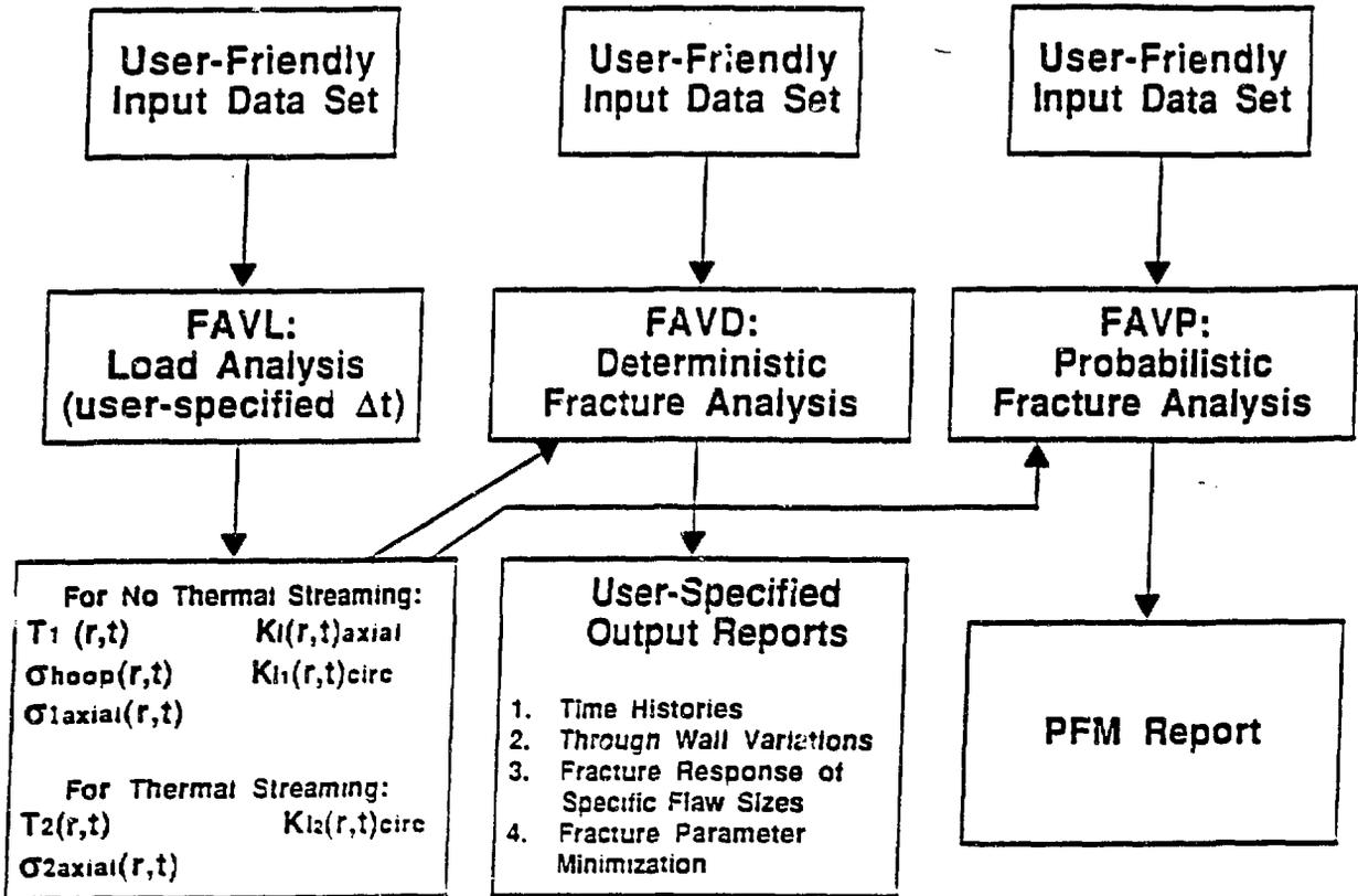
Figure 2. The FAVOR code is divided into 3 separate modules.
