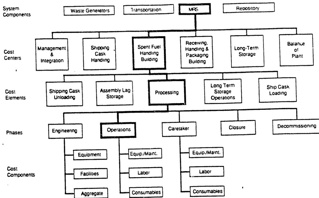
FIGURE 1 SYSTEMS ENGINEERING COST ANALYSIS MODEL (SECAM) - EXAMPLE COST ACCOUNTING STRUCTURE
