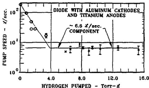
Figure 8. Hydrogen pumping speed of a diode sputter-ion pump with aluminum cathodes and titanium anodes.
