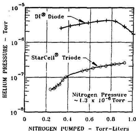
Figure 6. Helium partial pressure subsequent to pump regeneration and as a consequence of pumping nitrogen.
