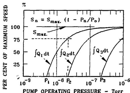
Figure 3. Increases in a capture pump's base pressure (i.e.,  $P_1$ ,  $P_2$  &  $P_3$ ) as a consequence of pumping increasing amounts of a particular gas (i.e.,  $\int Q_1 dt$ ,  $\int Q_2 dt$  &  $\int Q_3 dt$  respectively)
