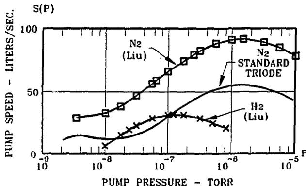
Figure 7.0. Nitrogen speed for a conventional triode sputter-ion pump and nitrogen and hydrogen speed for a triode pump with grided aluminum cathodes (Liu).<sup>(19)</sup>
