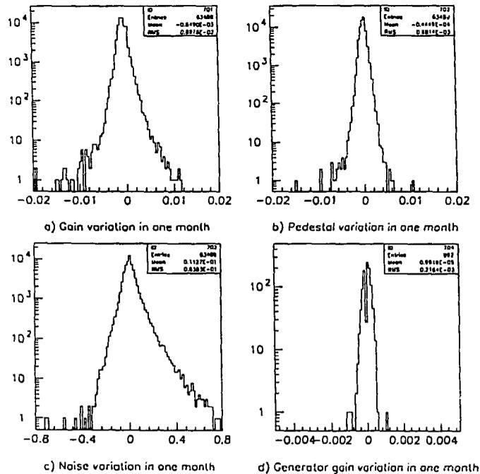
Figure 9: Relative variation of the calibration chain over one month
