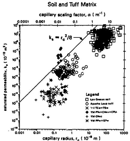
Figure 2 - Correlation between saturated permeability and capillary radius.
