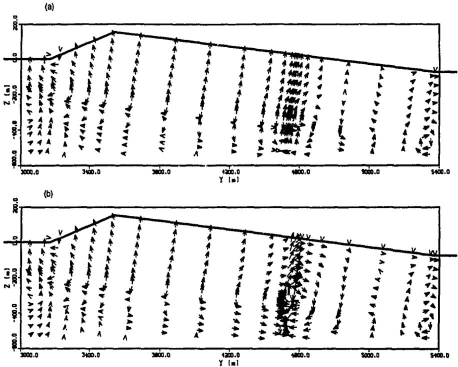
Figure 8 - The gas flow pattern at 100 year after waste emplacement for (a) reference case with no fault, (b) double-porosity representation of the fault.
