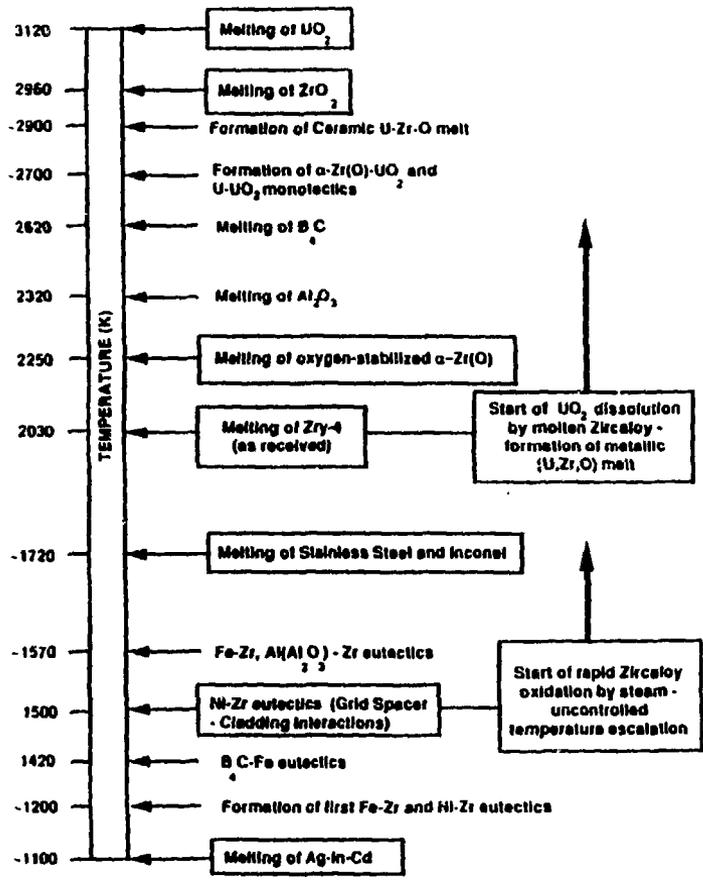
Fig. 2. LWR Severe Accident Relevant Liquid Phase Formation Temperatures
