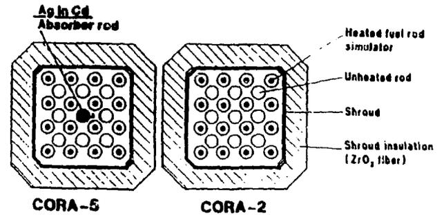
Fig. 3. CORA Experiment Configuration (PWR)
