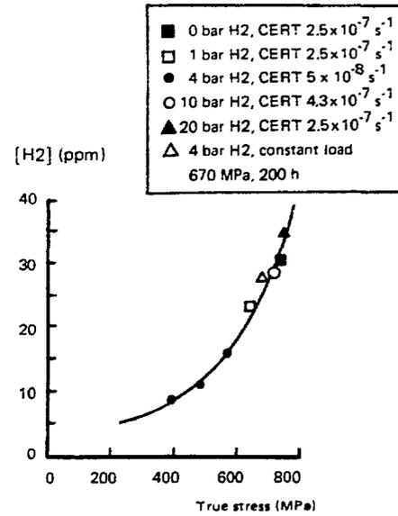
Figure 10 – Bulk hydrogen content as a function of the stress.
