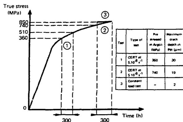
Figure 5 – Comparative crack depths during the slow propagation stage in CERT ( $5 \cdot 10^{-8} \text{ s}^{-1}$ ) and constant-load tests (tube 6L in the electro-polished conditions, primary water  $360^\circ\text{C}$ , 4 bar overpressure of hydrogen at  $125^\circ\text{C}$ ).
