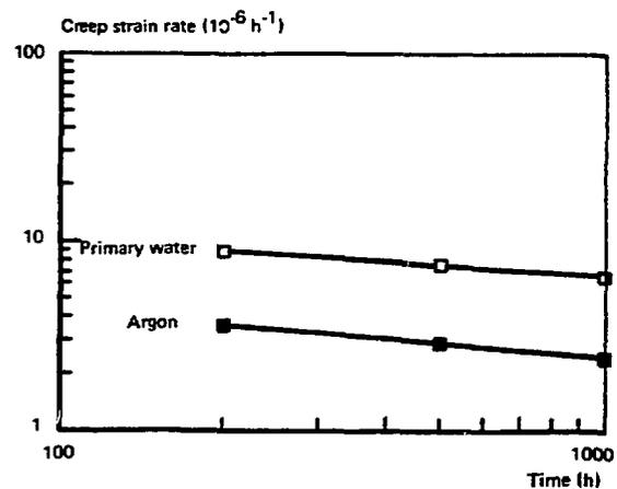
Figure 8 – Creep strain rate vs time for Alloy 690 in the electro-polished condition ( $360^\circ\text{C}$ , nominal stress: 600 MPa)
