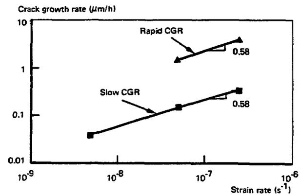
Figure 4 – Evolution of cracks growth rate as a function strain rate (tube 6.242R in the as-received condition, primary water 360°C, 4 bar-overpressure of hydrogen at 125°C).
