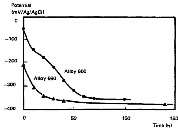
Figure 2 – Evolution of corrosion potential as a function of time (primary water without hydrogen, 350°C).
