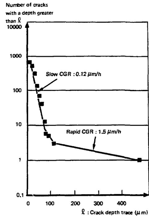
Figure 3 – Number of cracks with a trace depth greater than  $\ell$ , as a function of  $\ell$  (tube 6.242R in the as-received condition, CERT at  $5 \cdot 10^{-8} \text{ s}^{-1}$ , primary water 360°C, 4 bar-overpressure of hydrogen at 125°C).
