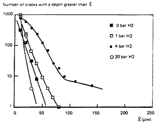
Figure 9 – Crack depth distributions; CERT ( $2.5 \times 10^{-7} \text{ s}^{-1}$ ); primary water  $360^\circ\text{C}$  with various hydrogen overpressures
