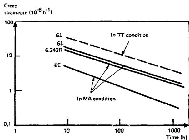
Figure 6 – Creep strain rate vs time, for three Alloy 600 tubes in the mill-annealed condition ( $360^\circ\text{C}$ , nominal stress: 650 MPa).
