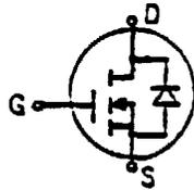
The drain is the positive electrode
