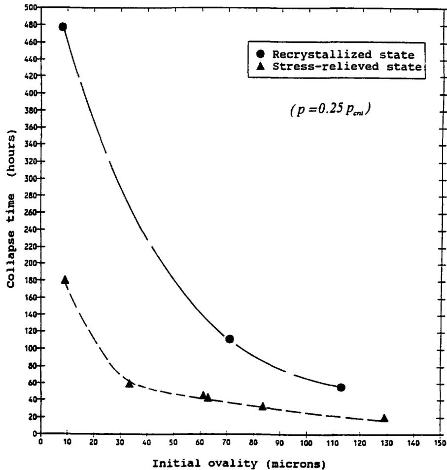
Fig. 2 Experimental collapse time as a function of initial ovality, under an external pressure of  $0.25 p_{crit}$
