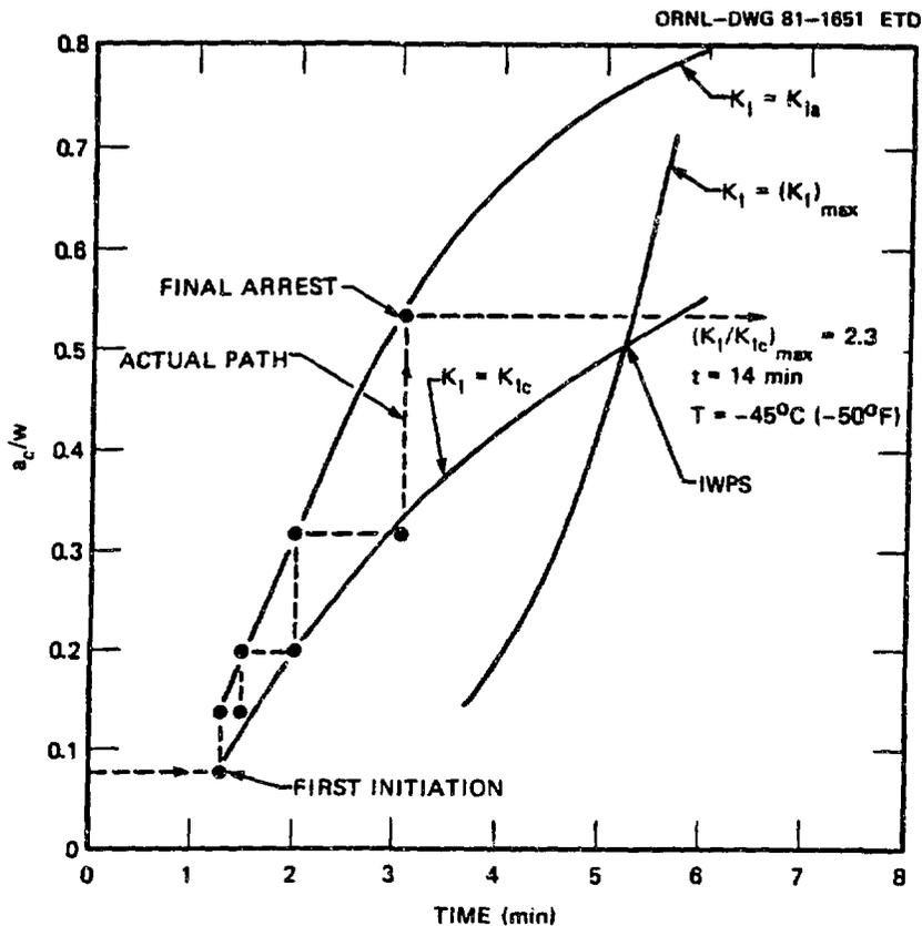
Fig. 15. Critical-crack-depth curves from posttest analysis of TSE-5A.
