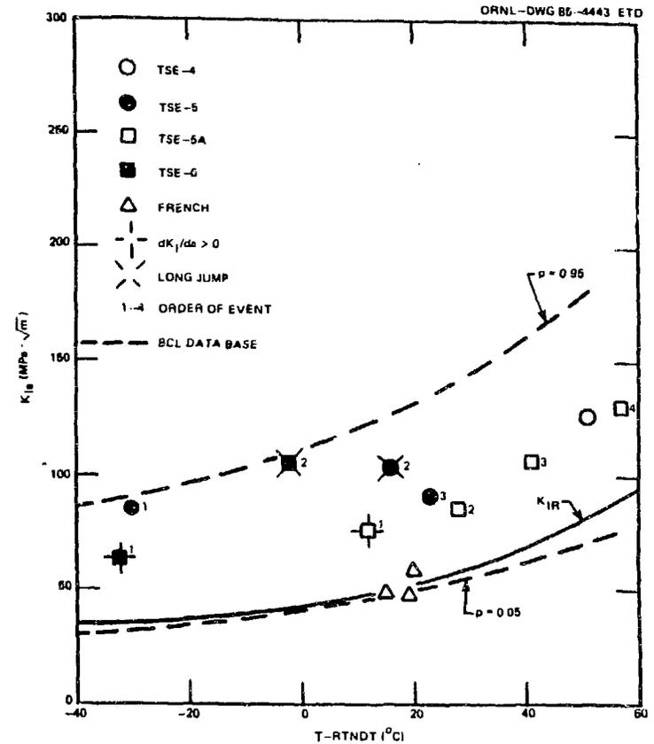
Fig. 19. Comparison of small-specimen and large-specimen  $K_{Ia}$  data.
