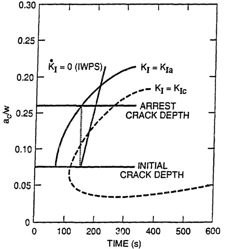
Fig. 11. Critical-crack-depth curves from posttest analysis of TSE-4.
