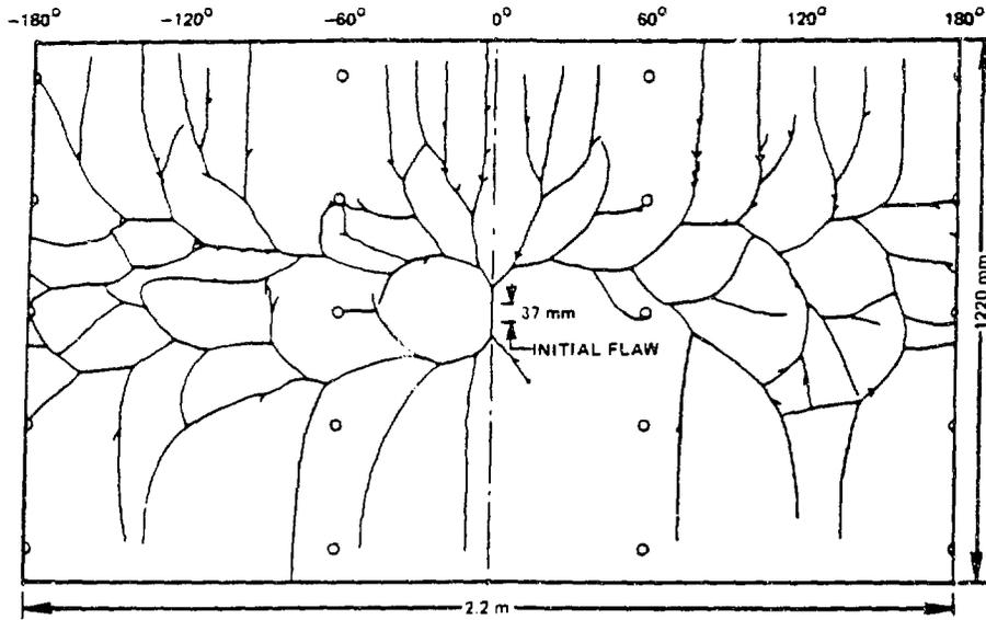
Fig. 20. Developed view of inner surface of TSE-7 test cylinder showing surface extension of initially small flaw (37 mm long x 14 mm deep).
