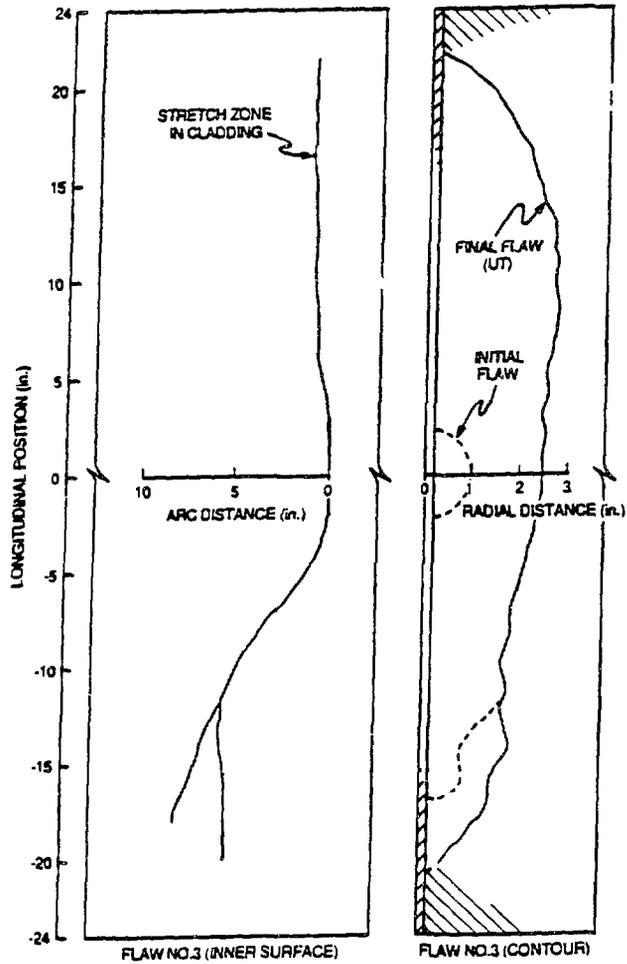
Fig. 22. Stretch-zone and ultrasonic-inspection indications of flaw 3 extension during TSE-8.
