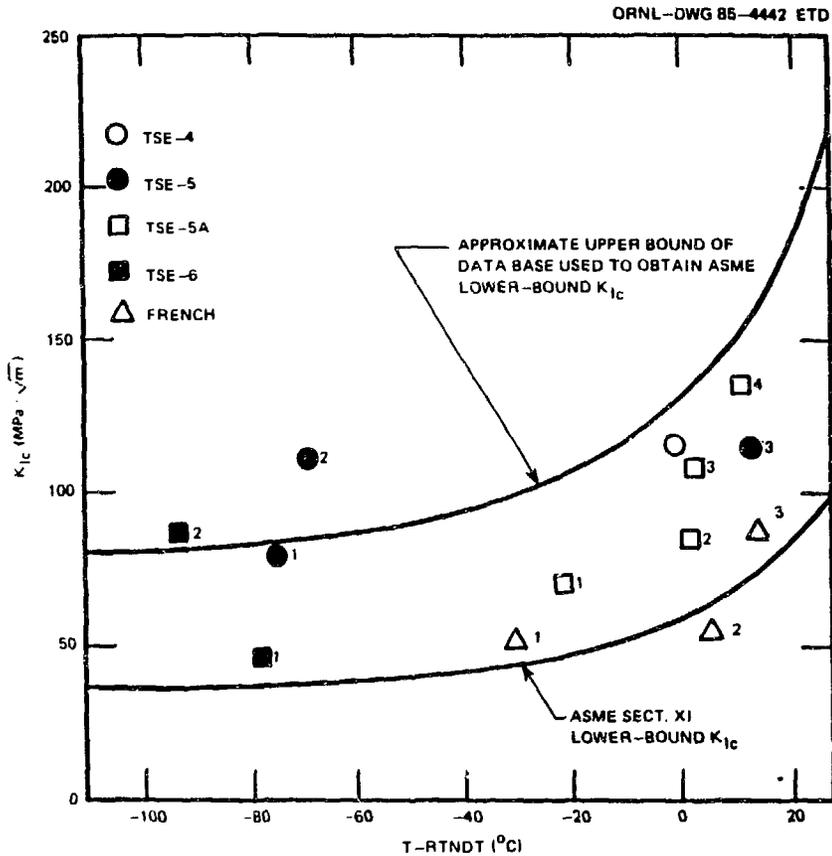
Fig. 18. Comparison of small-specimen and large-specimen  $K_{Ic}$  data.
