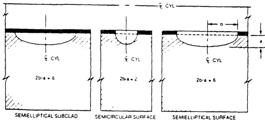
Fig. 7. Types of flaws for the clad-cylinder series of experiments
