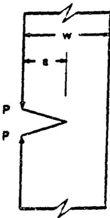
Fig. 3. Crack-mouth closing force associated with tensile stress in cladding over subclad flaw.
