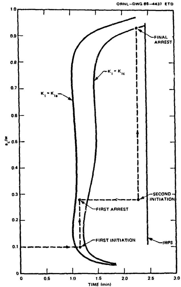
Fig. 17. Critical-crack-depth curves from posttest analysis of TSE-6.
