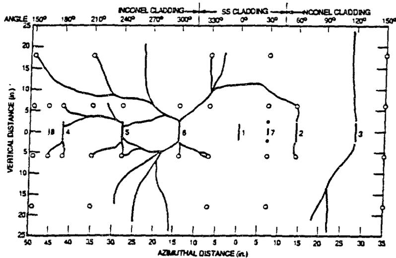
Fig. 23. Developed view of inner surface of test cylinder showing under-clad cracking pattern following TSE-11.
