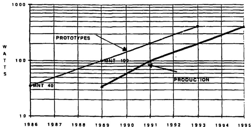
Dye lasers have been conceived by CEA and are experimented on specific laser chains at various repetition rates (Ref. 10). Fig 10 gives the development situation of qualified power amplifiers, this development being adjusted to pilot process facility needs.
