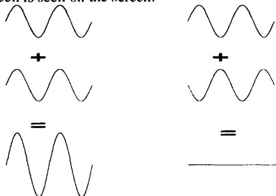
Fig. 2. Superposition of sine waves. The first two waves are in phase and the result is a wave with twice the amplitude. The other two are out of phase and the result is zero.
