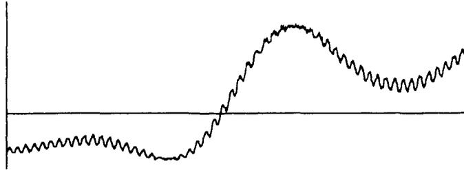
Fig. 3. Vibration measured with a Michelson interferometer. The small signal is a 5 kHz 15nm vibration from a piezo-electric transducer, the slow variations are changes in optical path in the interferometer arms due to background vibrations and temperature fluctuations.
