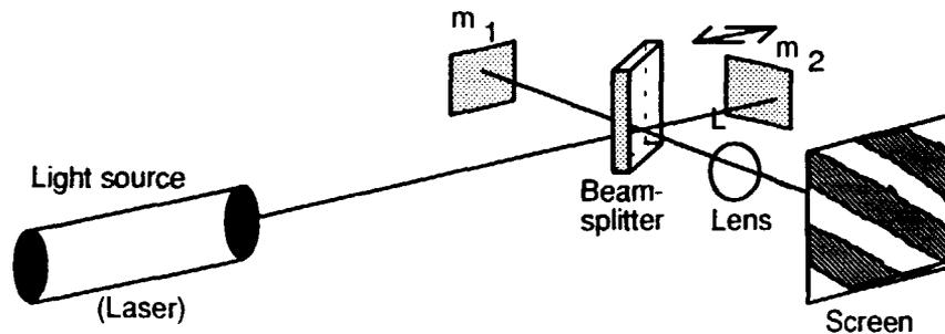
Fig. 1. Michelson interferometer.
