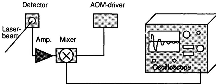
Fig. 8 Demodulation system.
