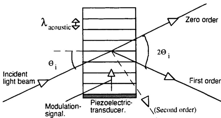
Fig. 24. Acousto optic modulator. Angles are exaggerated.
