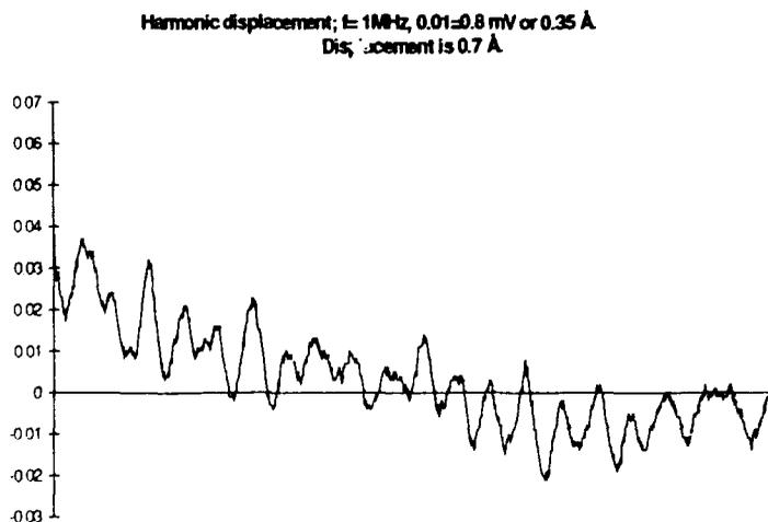
Fig. 20. Minimum detectable displacement, no averaging.
