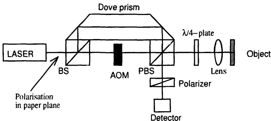
Fig. 21. An alternative interferometer set-up.
