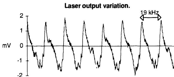
Fig. 18. Laser noise from voltage supply.
