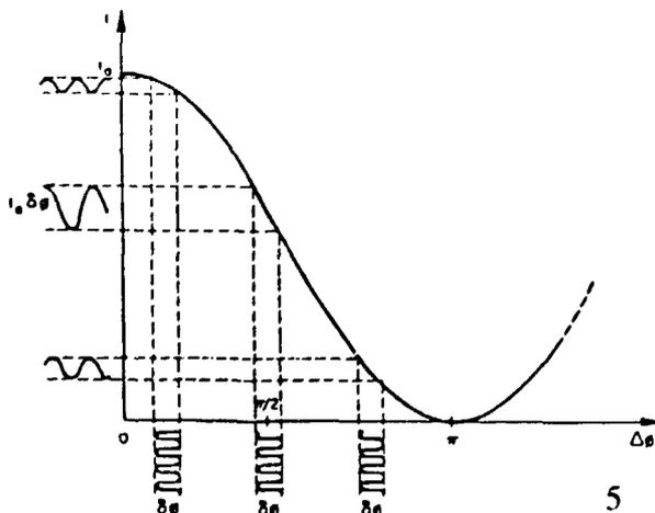
Fig. 4. The quadrature point in the fig. is when  $\Delta\phi$  is close to  $\pi/2$ . At the quadrature point the output signal caused by  $\delta\phi$  is large. When  $\Delta\phi$  is close to 0 or  $\pi$  the output signal is small. [from 4]. In the text,  $\theta$  corresponds to  $\Delta\phi$  and  $\varphi$  to the variation  $\delta\phi$ .
