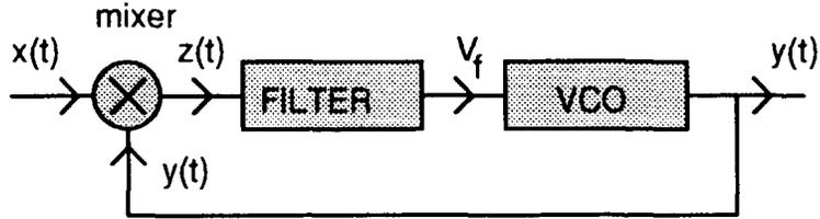
Fig. 23. Phase locked loop (PLL).
