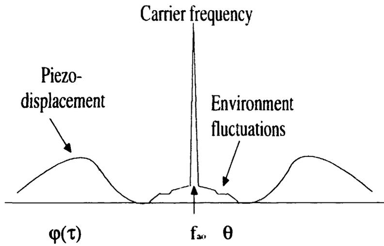
Fig. 7. Spectrum of detector signal with the carrier frequency  $f_{\omega_0}$  and the sidebands from the displacements,  $\varphi$ , and slow variations,  $\theta$ .
