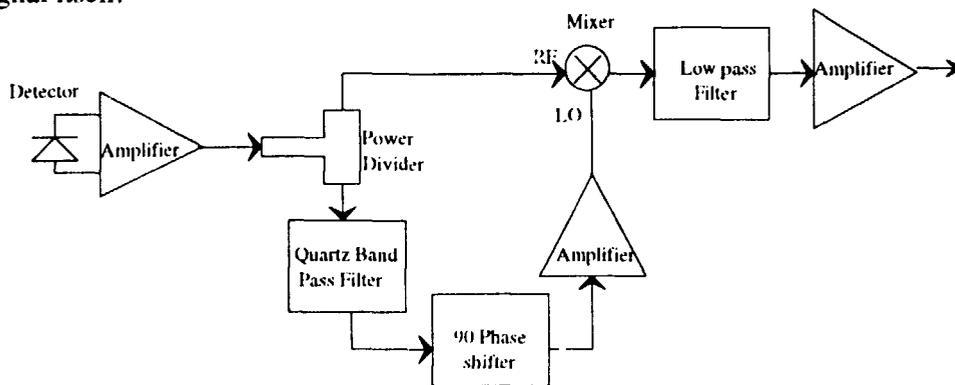
Fig. 22. Demodulation technique avoiding spurious vibrations.
