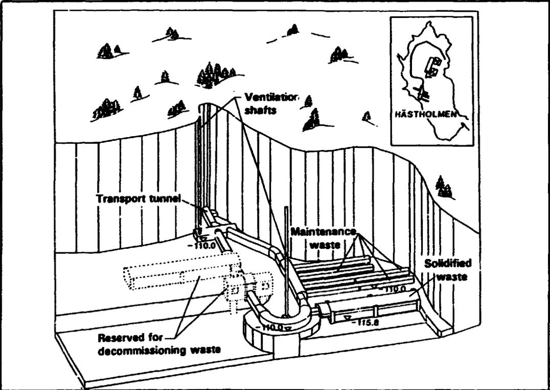
Fig 7. A diagram of a repository for low and intermediate level waste from the Loviisa nuclear power plant; the facility is being constructed on the island of Hästholmen.
