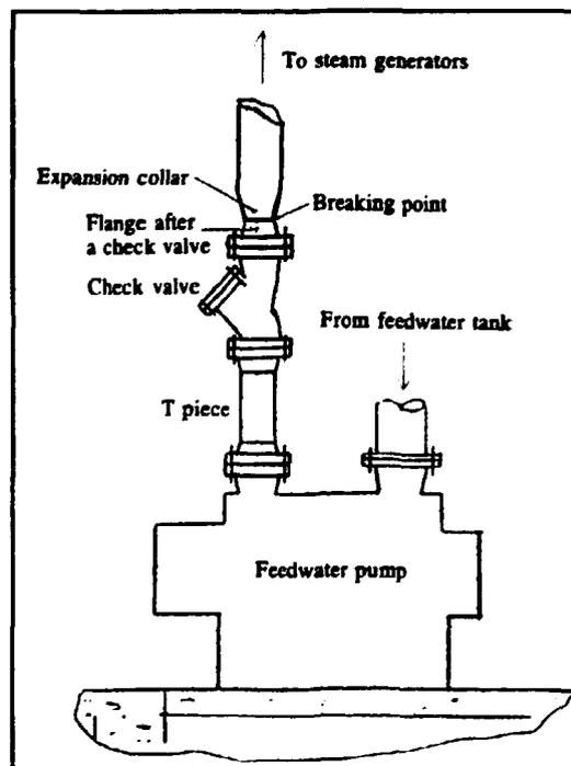
Fig 6. A diagram of the breaking point of a Loviisa feedwater pipe.
