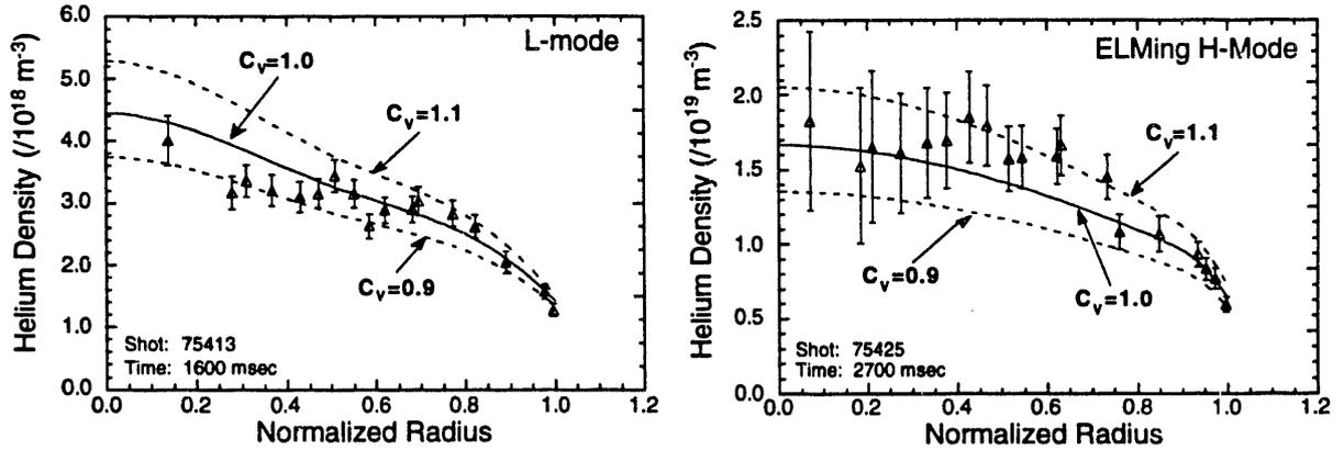
Fig. 1. Helium density profiles measured during L-mode and ELMing H-mode at  $I_p = 1.6$  MA along with curves showing the sensitivity to variation of the pinch coefficient  $C_v$ . The curve corresponding to  $C_v = 1.0$  is the normalized electron density profile inferred from Thomson scattering measurements.
