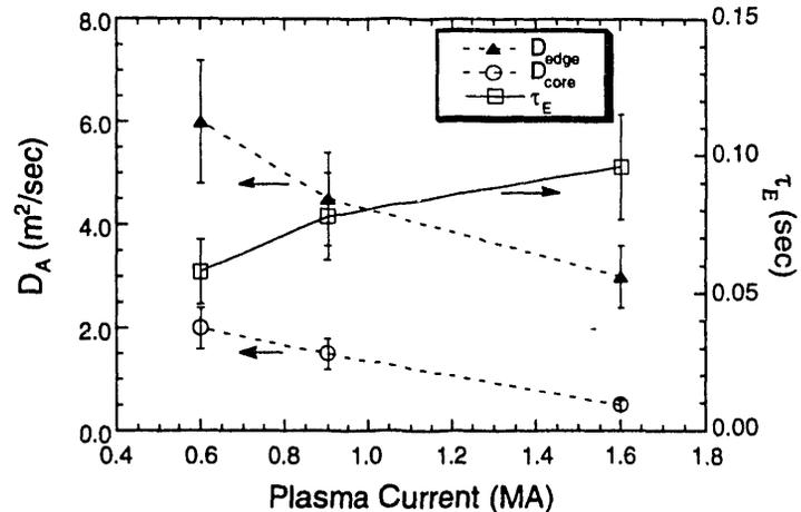
Fig. 2. Variation of diffusion coefficient and global energy confinement time with plasma current ( $P_{\text{NBI}}$  fixed at 10 MW).
