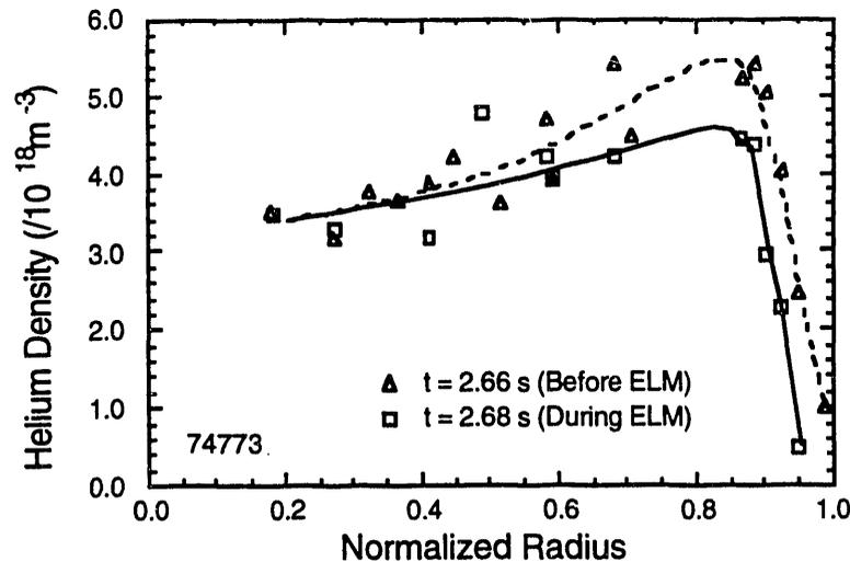
Fig. 3. Helium density profiles measured by just before and after a giant ELM event during a 1.6 MA H-mode discharge.
