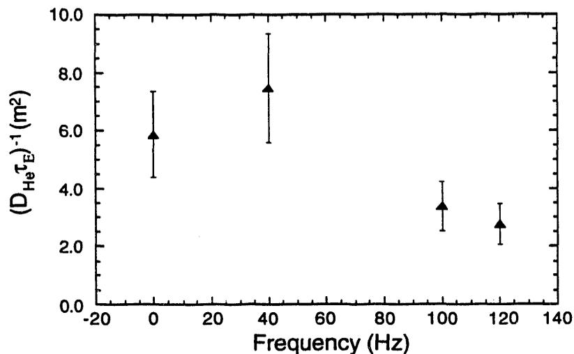
Fig. 4. Scaling of the parameter  $1/(D_A^\alpha \tau_E)$  as the ELM frequency is varied from 0 Hz (ELM-free) to 120 Hz.
