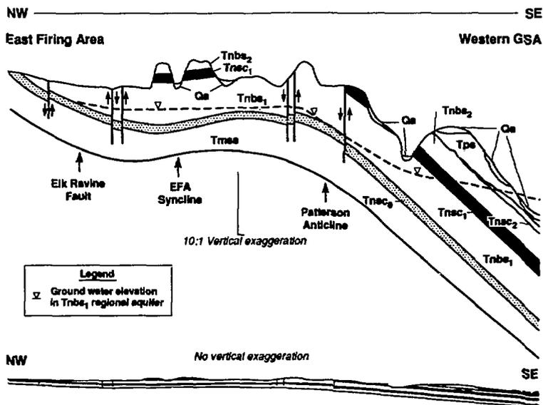
Figure 5. Generalized cross section of Site 300.
