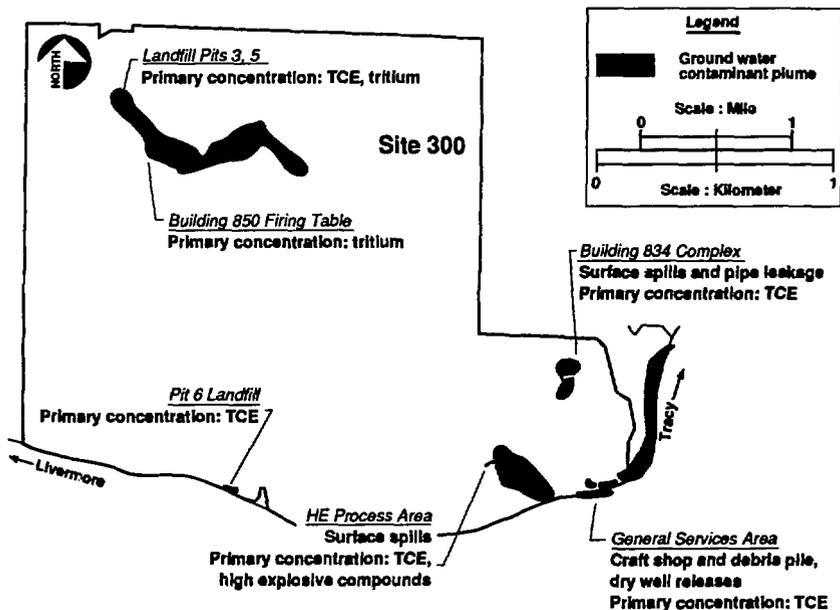
Figure 2. Release points and extent of contaminants in ground water at LLNL Site 300 and offsite areas.
