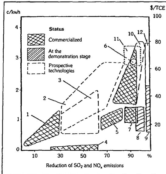
Fig. 7. A comparison between costs and efficiencies of various emission control measures [EPRI assessment with author's additions]
