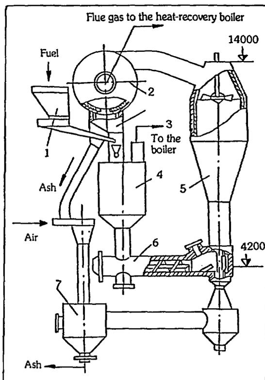
Fig. 3. Layout of the ENIN combustor module
