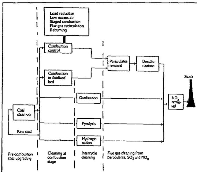
Fig. 1. Different emission control options
