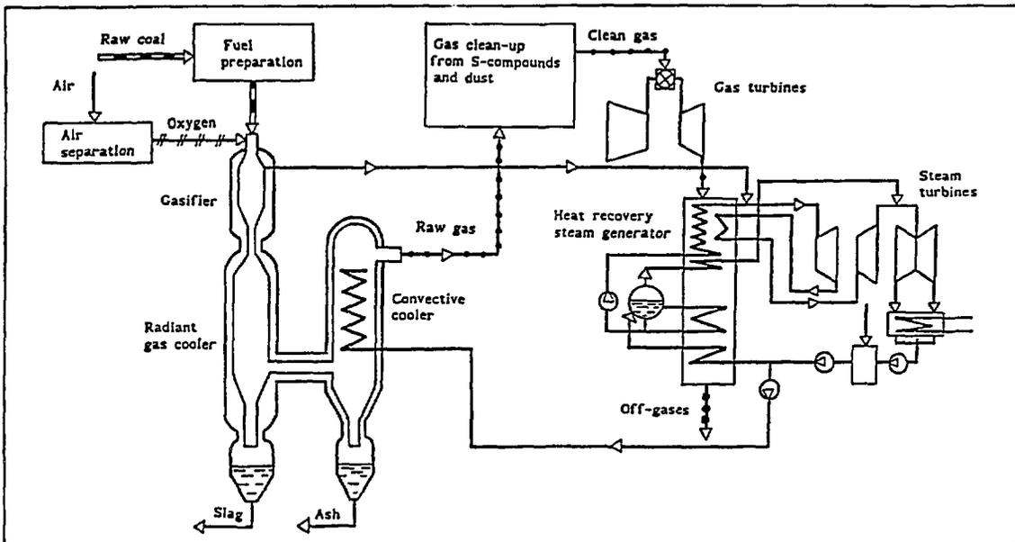
Fig. 5. Principal scheme of the 625 MW IGCC unit (Berezovsky Plant-2)
