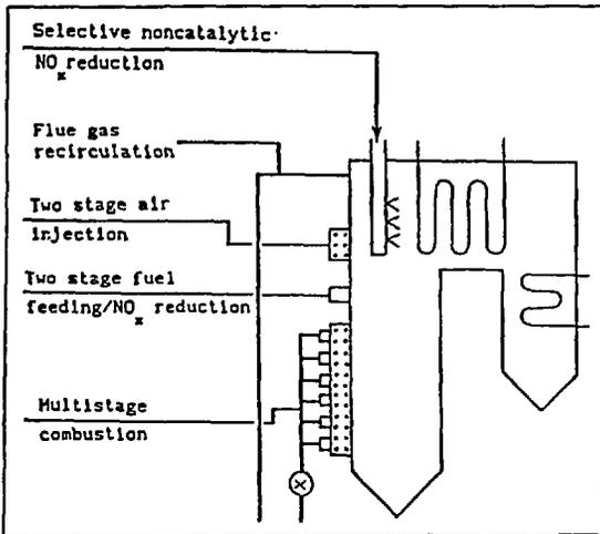
Fig. 4. Methods for  $\text{NO}_x$  control at the combustion stage
