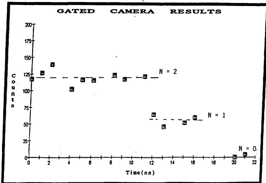
Fig. 3. Gated camera results from SSRL show observation of single electron bunch ( $N=1$ ) is possible with visible synchrotron radiation.
