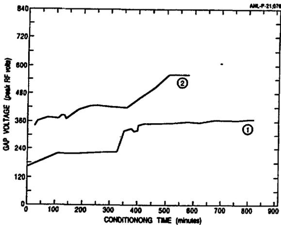
Figure 2 - Multipacting conditioning behavior of a niobium multipacting test cavity at 4.2 K. Multipacting level as a function of conditioning time is shown for (1) the initial cooldown and (2) after warming to room temperature for several days without exposure to air. During conditioning, typically 1 watt was coupled into the cavity.
