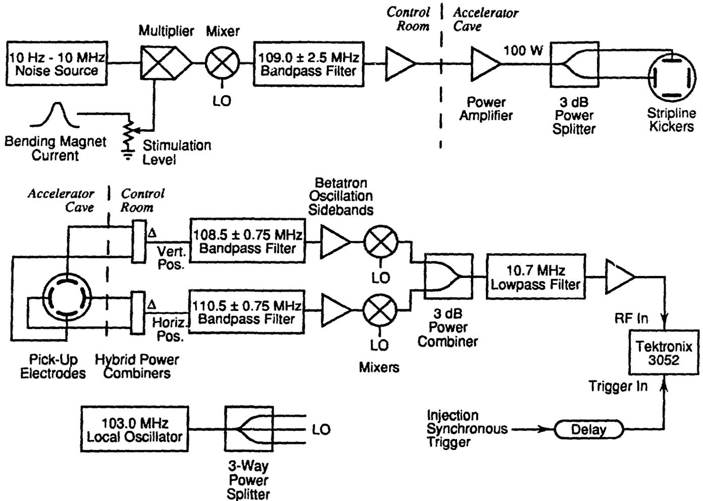
Fig. 1. NSLS booster tune measurement system block diagram.
