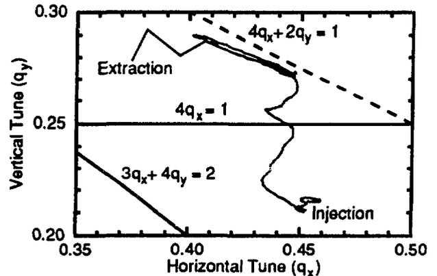
Figure 3. Horizontal vs. vertical tune in the NLS booster obtained from the data in fig. 2, smoothed to eliminate rapid oscillations. The third and fourth order resonance lines in this region of the tune plane are indicated.
