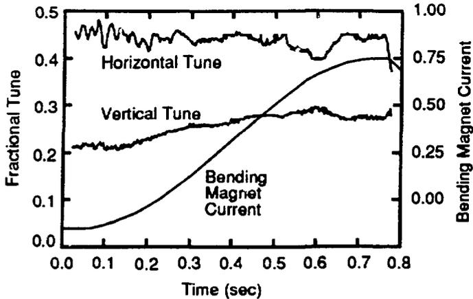
Figure 2. Horizontal and vertical tunes in the NLS booster as a function of time during the acceleration cycle. Also shown is the booster bending magnet current which is proportional to beam energy.
