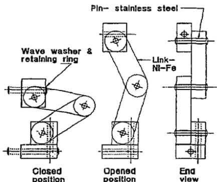
Figure 3. Flux shunt linkage.
