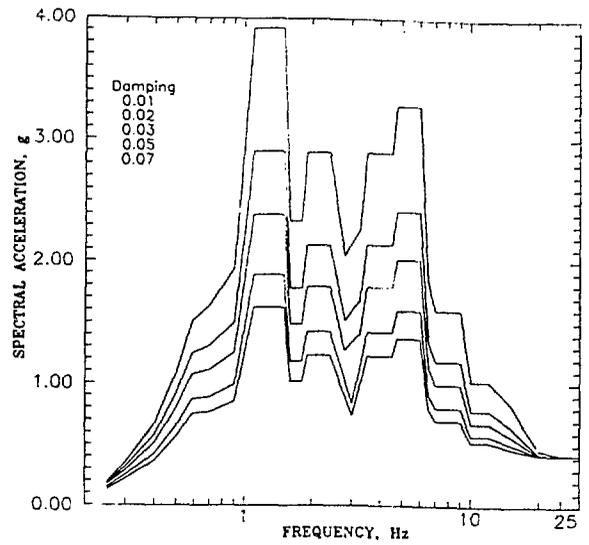
Fig. 6 Floor Spectrum at Level of 28.4 m of the Intermediate Building
