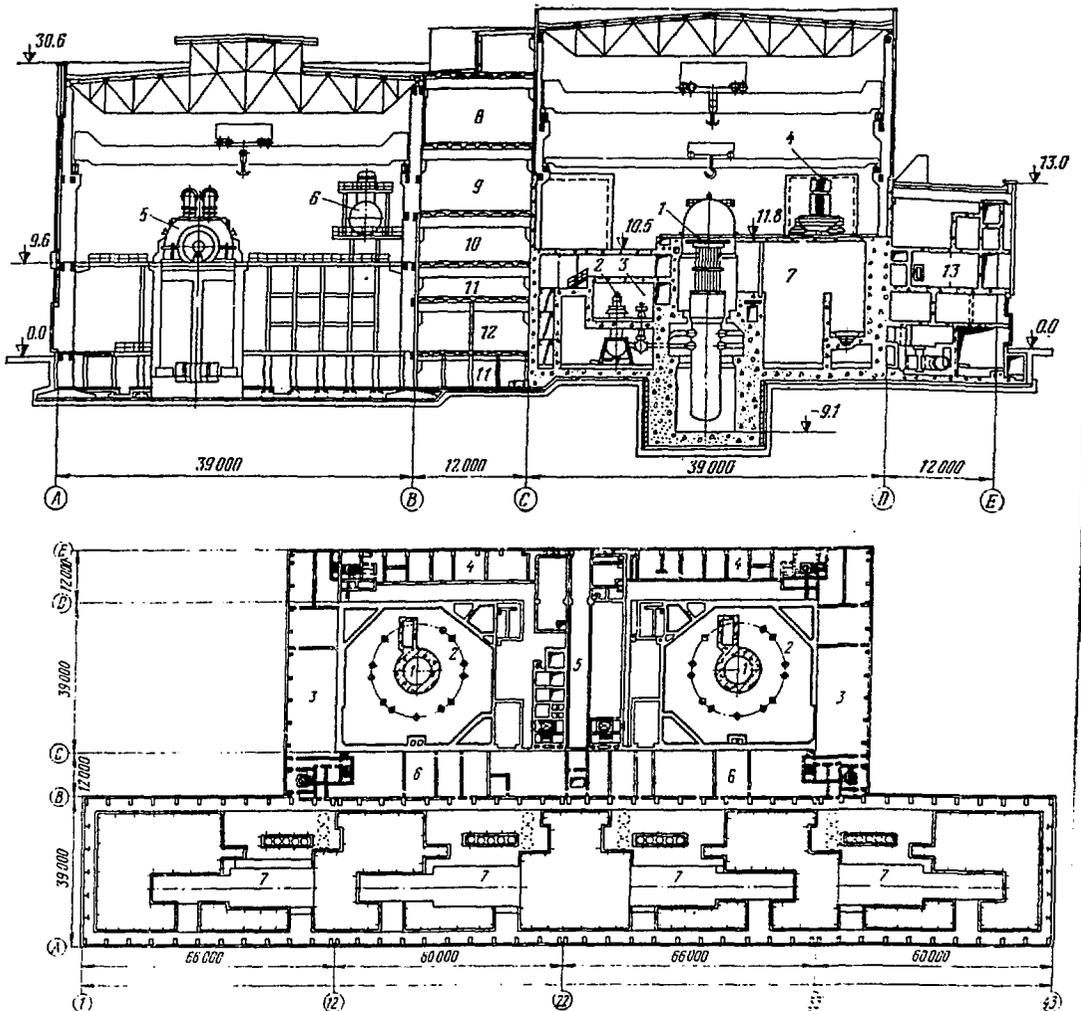
Fig. 2 Elevation and Plan Views of the Main Building
