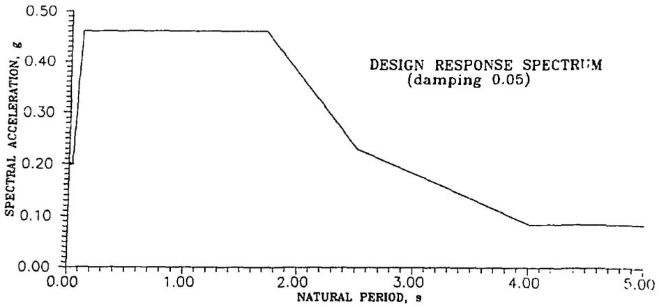
Fig. 1 Site Ground Spectrum (5% damping)
