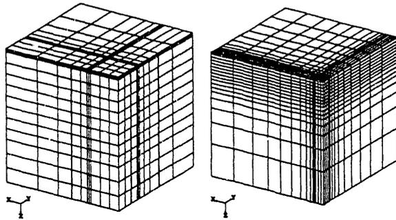
Figure 2. Finite element meshes for heatup and cooldown
