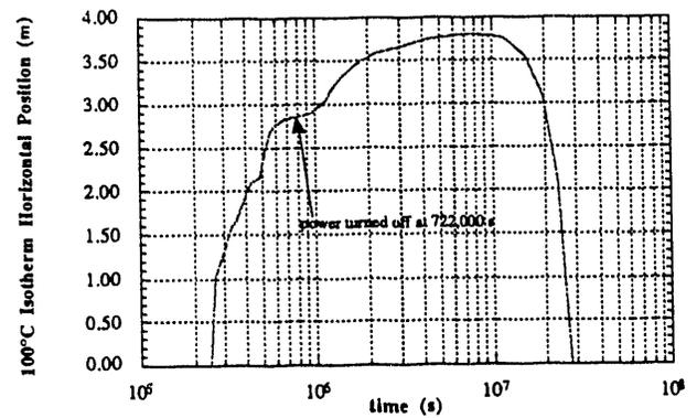
Figure 12. 100°C isotherm horizontal position at 1.94 m depth vs. time.
