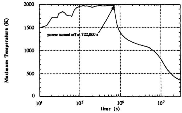
Figure 5. Maximum temperature in melt.
