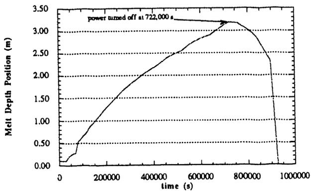
Figure 9. Melt depth position in center of melt vs. time.
