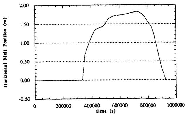
Figure 10. Horizontal melt position at 1.94 m depth vs. time.
