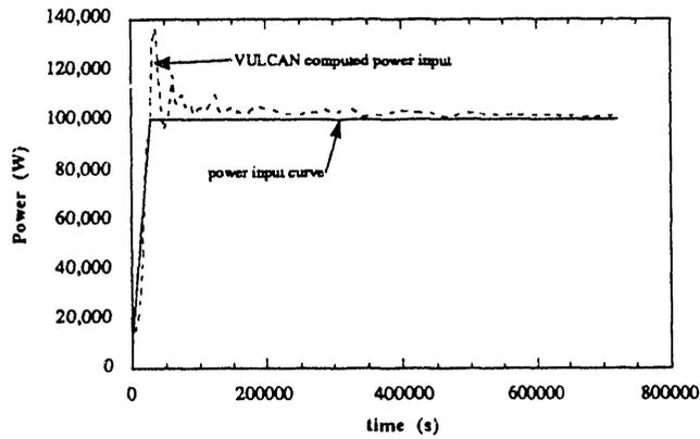
Figure 3. VULCAN computed power vs. power input curve.
