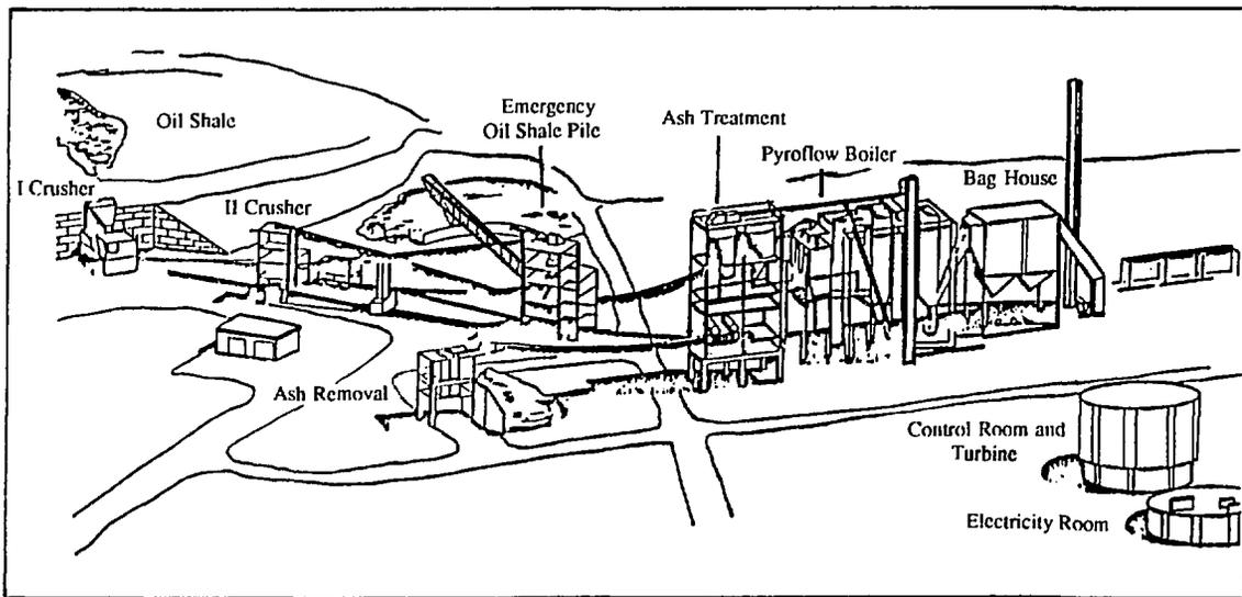
Fig. 6. Overview of the demonstration plant for direct combustion of oil shale
