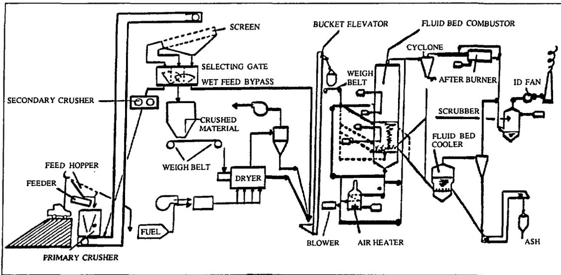
Fig. 5. PAMA's fluidized bed combustion pilot plant
