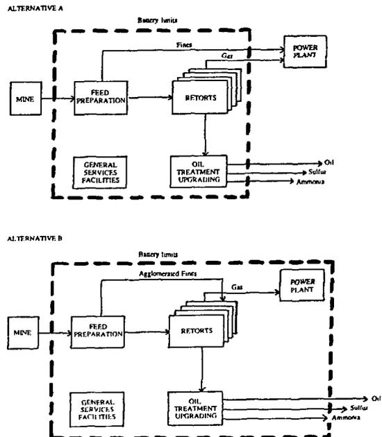
Fig. 3. Alternatives for oil production by oil shale retorting
