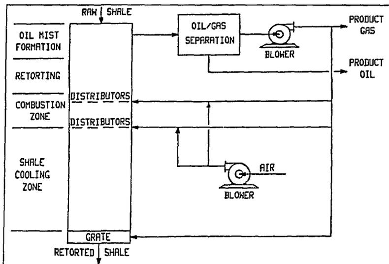
Fig. 2. Moving bed retort — directly heated
