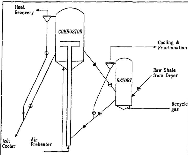
Fig. 4. Simplified scheme of fluidized bed retort and combustion system
