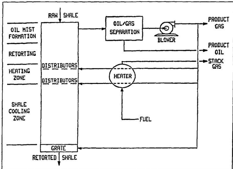
Fig. 1. Moving bed retort — indirectly heated
