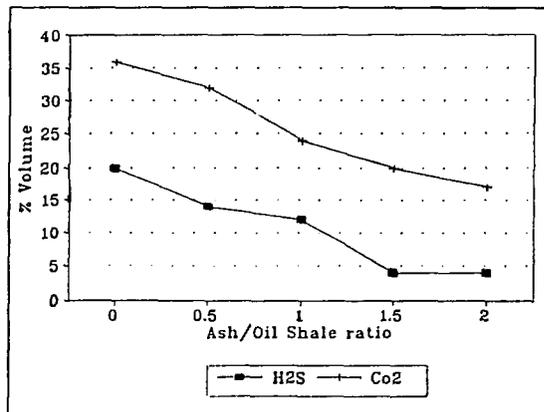
Fig. 6. Gas composition at different ash/oil shale ratios
