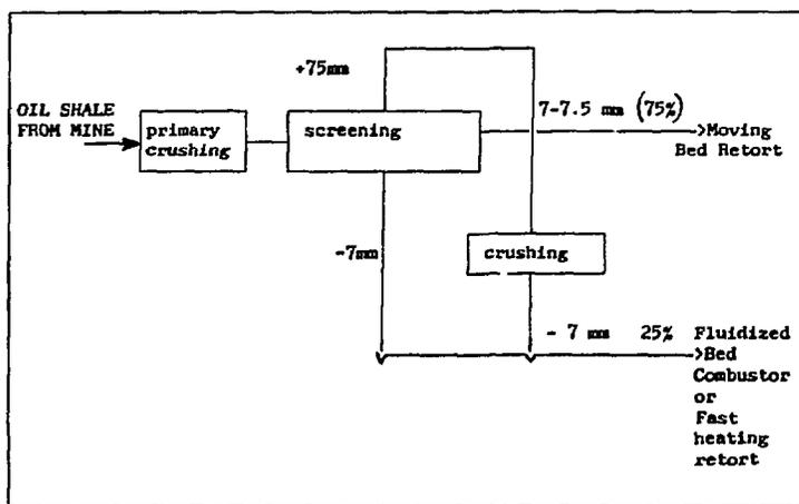
Fig. 3. Integration of moving bed retort and oil shale fines utilization
