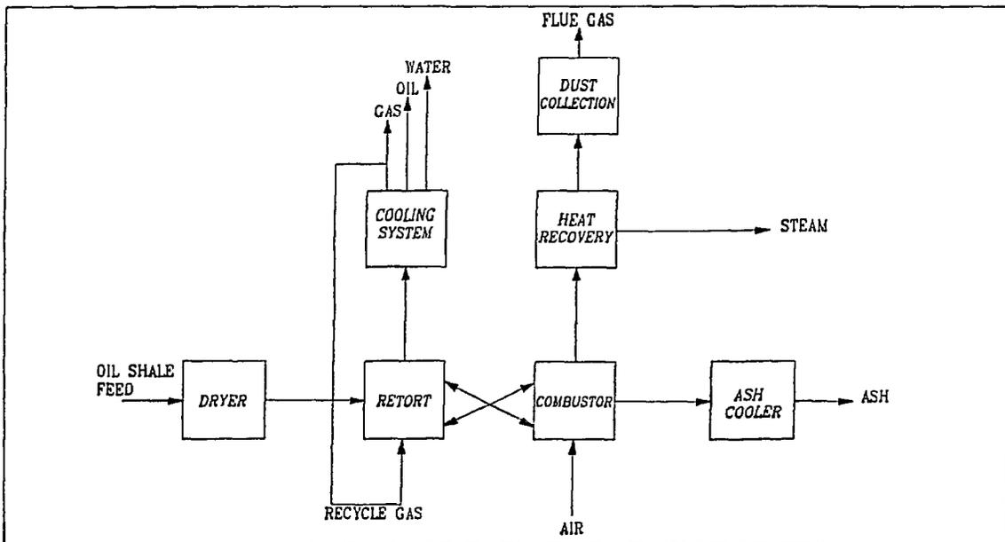
Fig. 5. Block diagram of fast heating retort process
