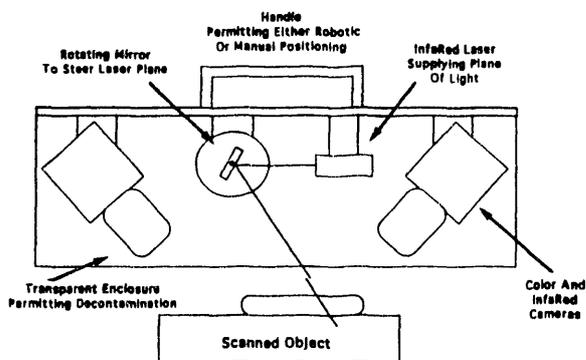
Fig. 5. SCOPE schematic
