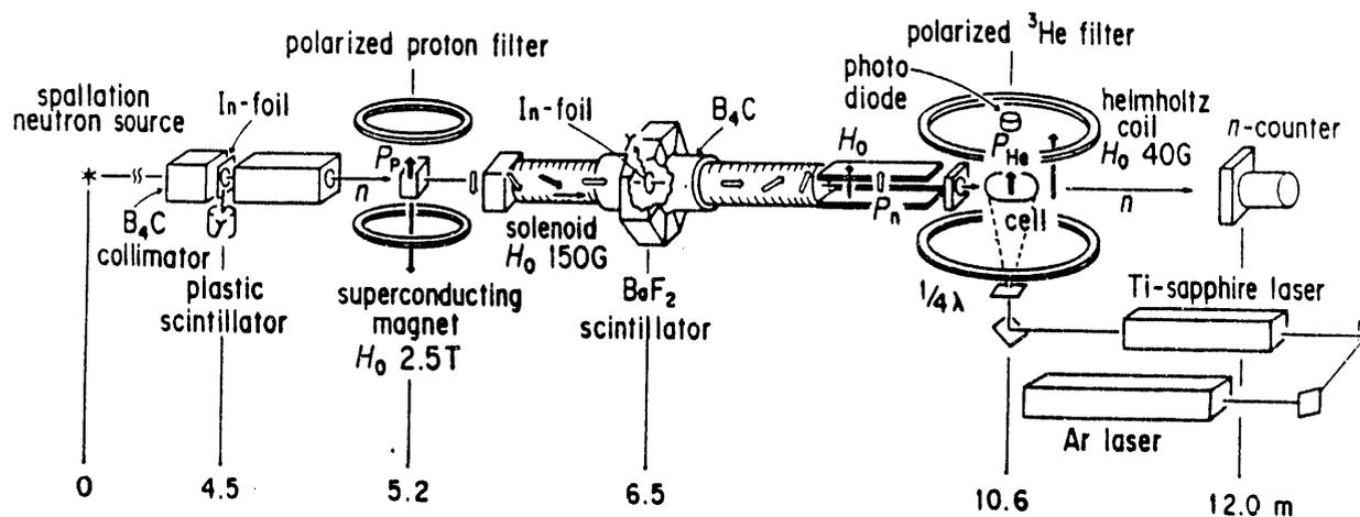
Fig. 1 Polarized  $^3He$  neutron polarimeter.
