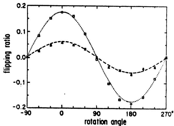
Fig. 3 Flipping ratio of the polarized  $^3He$  transmittance as a function of  $\theta$ .
