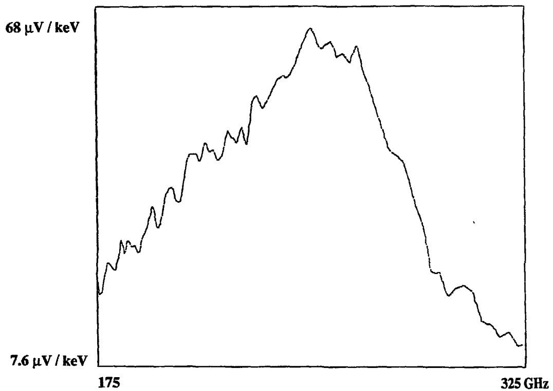
Fig.4 Calibration spectrum ( 80 frequency points - 50 mn integration time per point )
