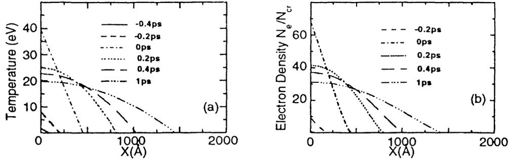
FIG.3: (a) Calculated electron temperature profiles at different instants as predicted by the nonlinear heat wave model. The simple approximate method to the Saha equations<sup>10</sup> is used to estimate (b) the corresponding electron plasma density profiles in the bulk target.
