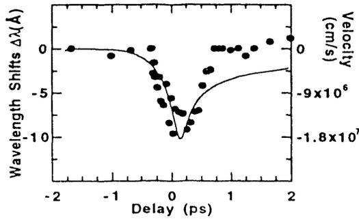
FIG.2: Wavelength shifts (close circles) in the enhanced reflected backside probe light are observed during the first picosecond after the pump pulse. Solid curve is calculated shifts from the nonlinear heat wave model.
