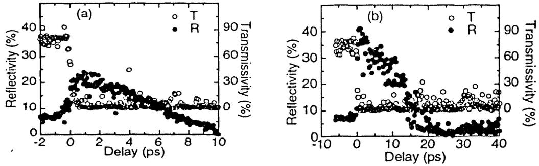
FIG.1: Simultaneous scans of single-shot reflection (close circles) and transmission (open circles) of (a) the frontside probe and (b) backside probe pulses are measured as functions of time delay between the strong pump and weak probe pulses.
