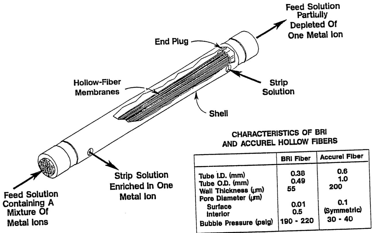
Figure 2. CT Hollow-Fiber Modules
