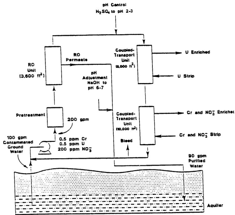
Figure 1. RO/CT Hybrid System for Groundwater Remediation
