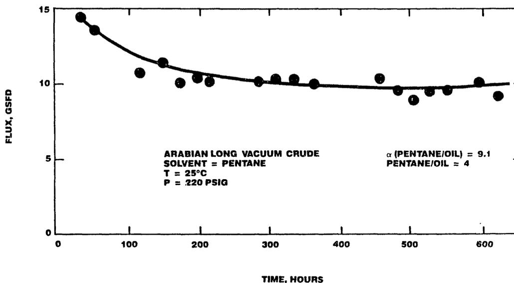
Figure 2. Long-Term Performance of Module for Solvent Recovery
