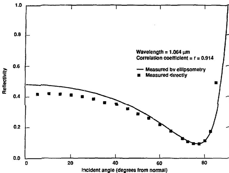
Fig. 2. A comparison of measurements of the parallel polarized reflectivity of Highly Ordered Pyrolytic Graphite (HOPG)
