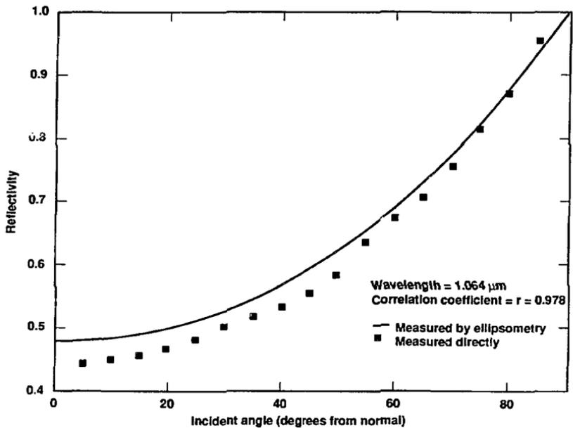
Fig. 3. A comparison of measurements of the perpendicularly polarized reflectivity of Highly Ordered Pyrolytic Graphite (HOPG)
