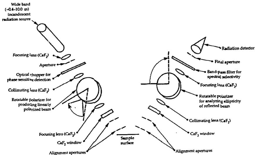
Fig. 1. Schematic of the ellipsometry measurement system.
