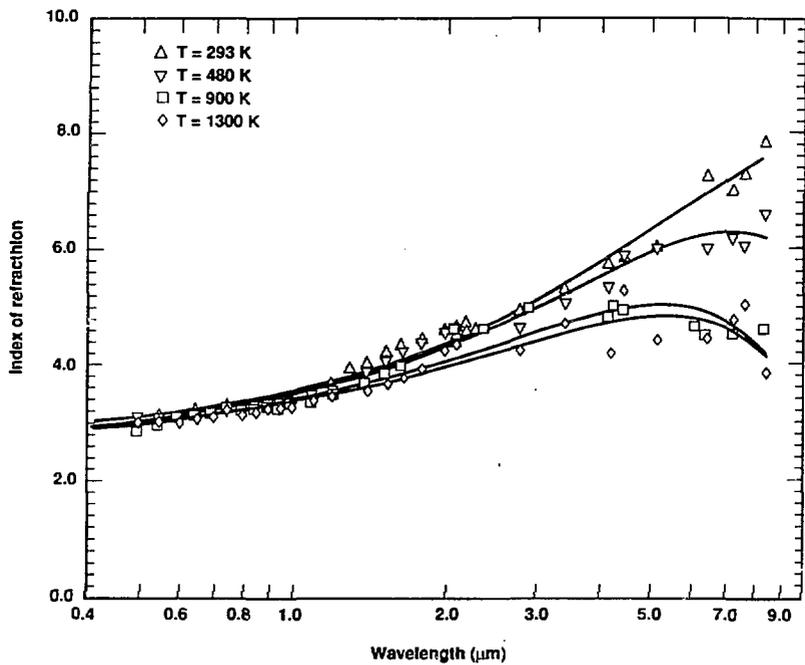
Fig. 5. The Index of refraction of HOPG.
