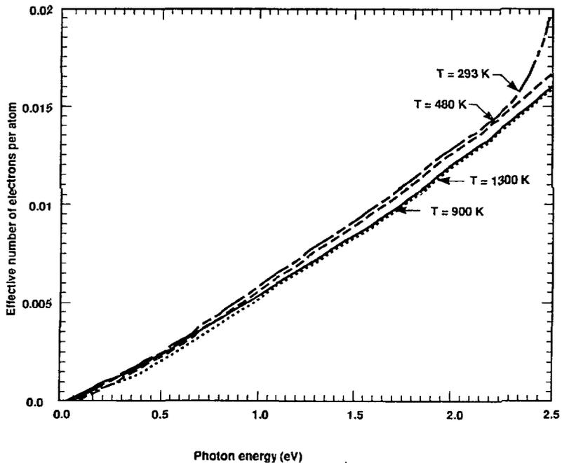
Fig. 9. The effective number of electrons per atom versus photon energy obtained from integration of curve fits to the results for conductivity.
