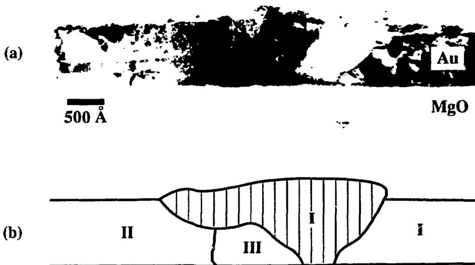
Fig. 3. (top) Cross-sectional TEM view of the Au portion of an ion-beam mixed Au/Cu bilayer containing a DIGM alloyed zone. (bottom) Schematic of above micrograph with hatched region delineating the DIGM alloyed ( $\geq 20$  at. % Cu) zone. Different Au grain orientations indicated by I, II, and III.
