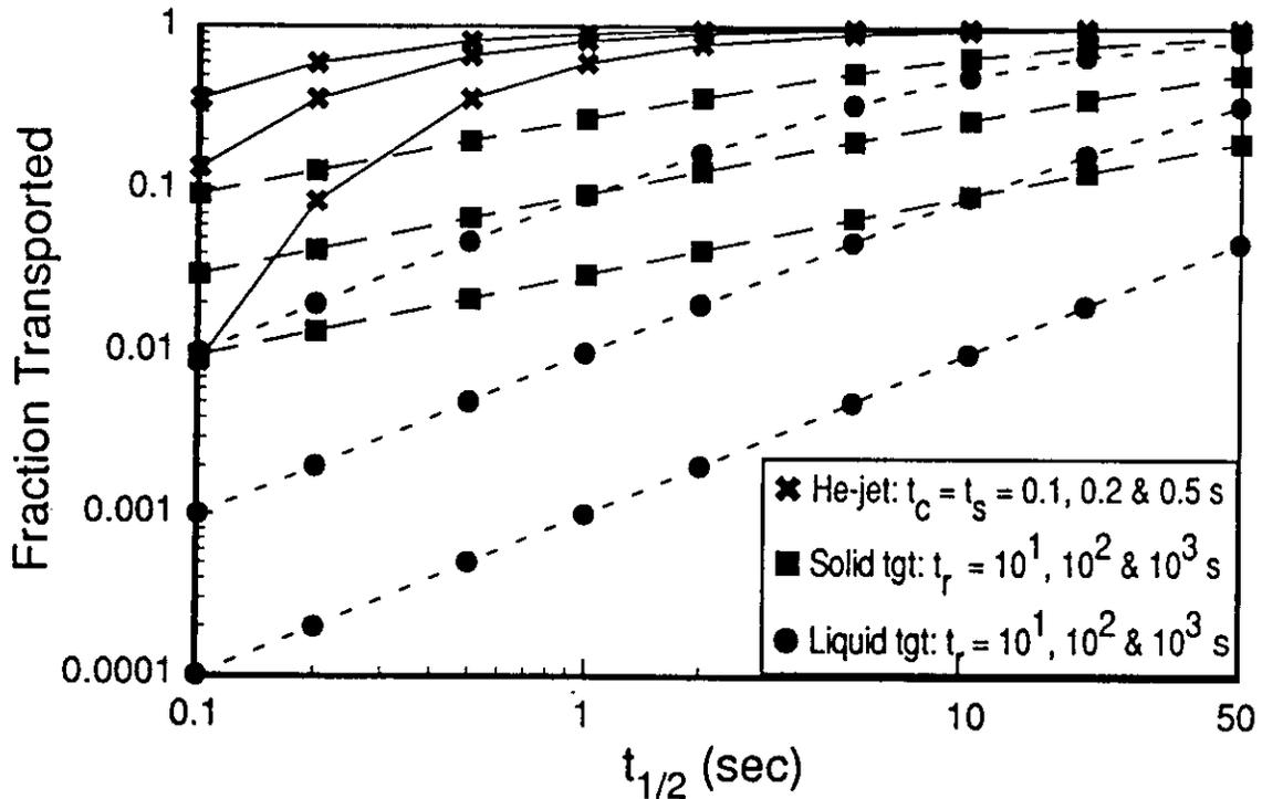
Fig. 1: Fraction of activity transported (released) versus half-life for a thin-target, He-jet system compared to two types (solid and liquid) of thick target, integrated ion source systems ( $t_c$  = capillary transit time,  $t_s$  = sweep out time of the target chamber,  $t_r$  = release time from thick target). Taken from Ref. 5.
