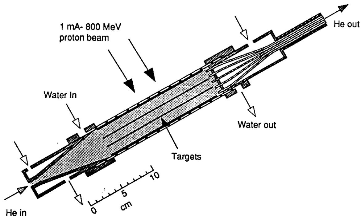
Fig. 2: Sketch of the LAMPF He-jet target chamber.
