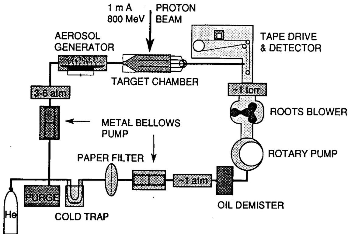
Fig. 3: Schematic of the He-jet gas recirculation system.
