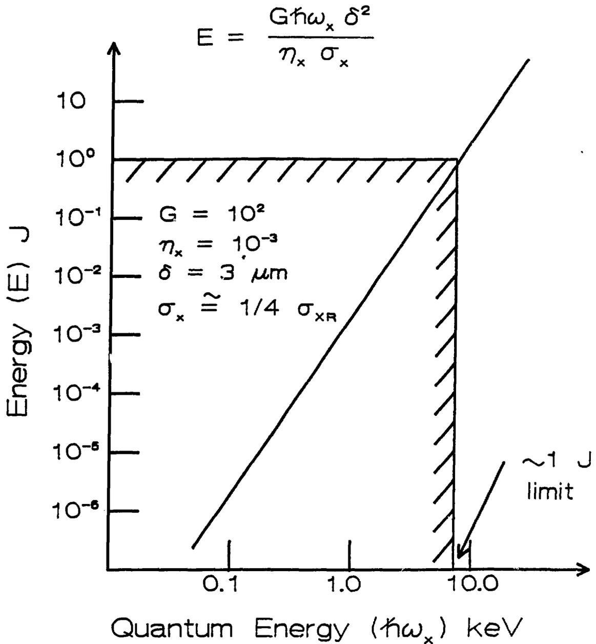
Fig. 1: Scaling relationship between required excitation energy (E) and quantum energy ( $\hbar\omega_x$ ) characteristic of the amplifier. Parameters: total gain exponent  $G = 100$ , energy efficiency  $\eta_x = 10^{-3}$ , channel diameter  $\delta = 3 \mu\text{m}$ , x-ray ( $\hbar\omega_x$ ) cross section for stimulated emission  $\sigma_x$ , x-ray cross section for stimulated emission for radiatively-broadened transition  $\sigma_{xR}$ .
