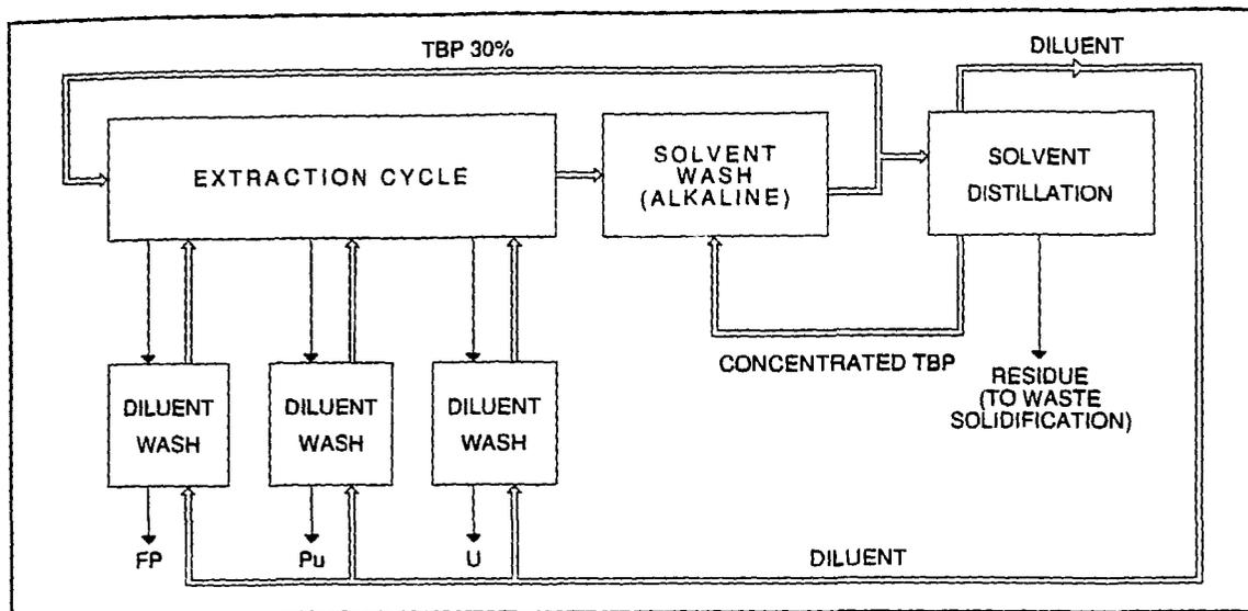
Figure 4: Solvent Management Diagram
