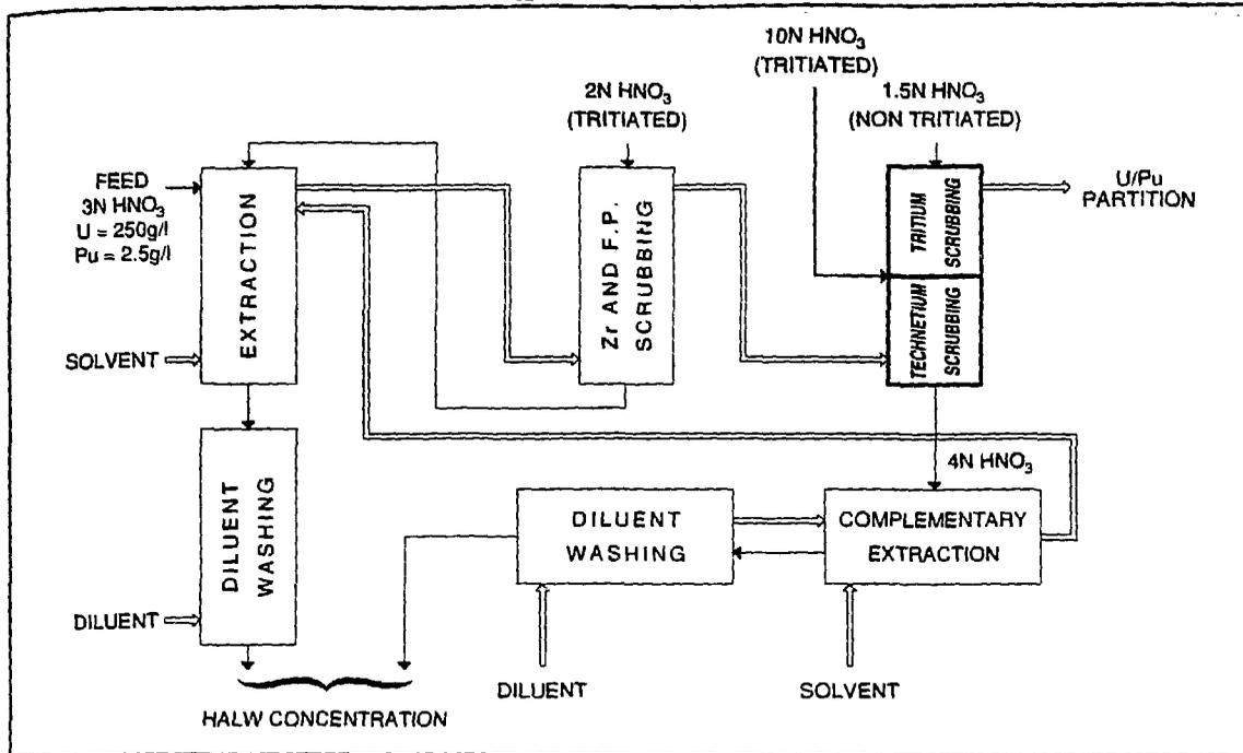
Figure 3: First Extraction Cycle: Technetium and Tritium Scrubbing
