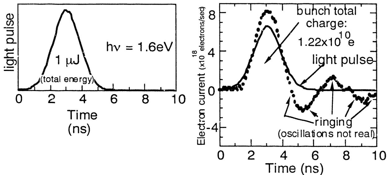
Figure 2. A light pulse with the corresponding electron bunch.
