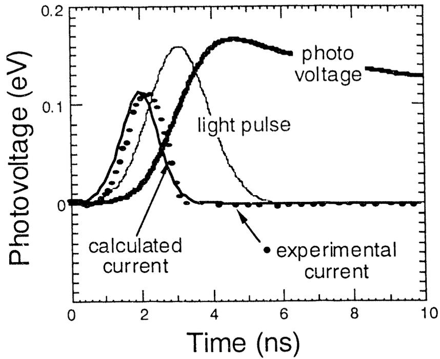
Figure 12. Photovoltage as a function of time. Also shown are the experimental and calculated electron response, as well as the light pulse.
