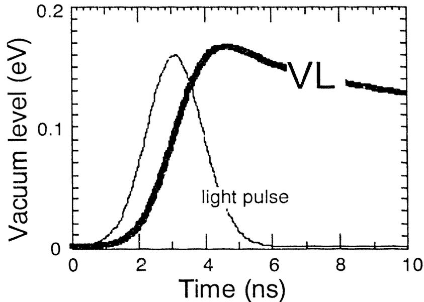
Figure 7. Calculated vacuum level rise when illuminated with a high-intensity light pulse of  $65 \mu\text{J}$  total energy. After the light is gone, the VL comes back to its original position. This is due to the restoring mechanism that will be explained in the next section. The effect shown in Fig. 4 can be easily explained by noticing that the VL remains up for a period of time.
