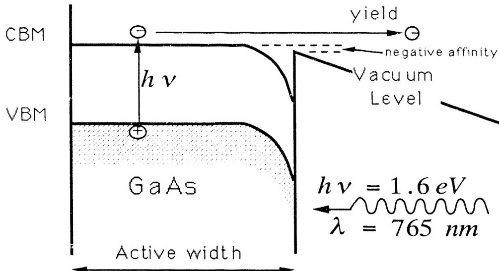
Figure 1. A simplified schematics of the SLAC cathode.
