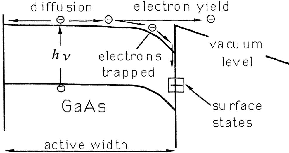
Figure 5. A schematic of the photoemission process in the SLAC cathode.
