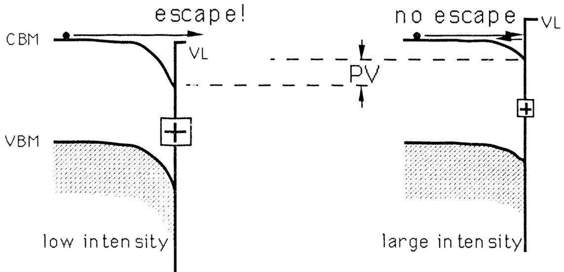
Figure 6. In the low intensity case (left), the surface charge and band bending are large, so VL is low and the electrons can escape easier. With high light intensity (right), there are many electrons falling into the surface states, decreasing the amount of positive charge at the surface, so the band bending decreases. This process raises the vacuum level (VL), so that electrons reaching the surface find a larger barrier to escape.
