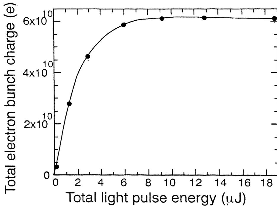
Figure 3. There is a limit on the total amount of electrons obtainable from the cathode. This is the Charge Limit (CL) effect.
