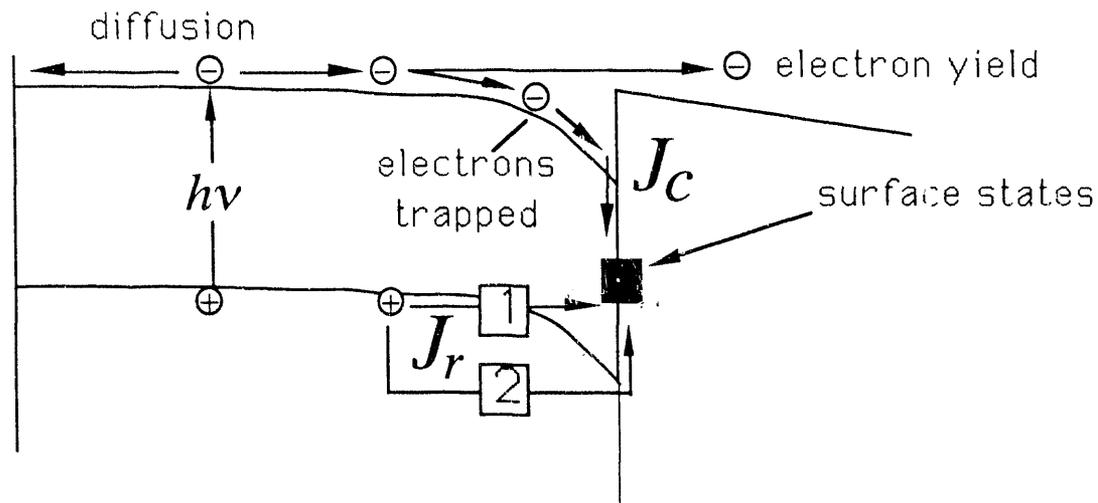
Figure 10. Electrons trapped at the surface of a heavily doped p-type semiconductor can tunnel and recombine. The trajectory mark with "1" is the hole tunneling current ( $J_{\text{tunn}}$ ), and with "2" is the thermionic emission current ( $J_{\text{th}}$ ). The  $J_C$  is the current from the photoexcited electrons in the conduction band into the surface, and  $J_r$  are the restoring currents.
