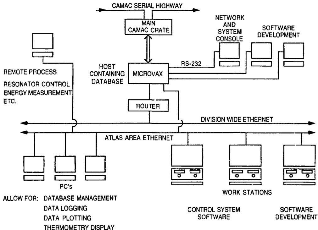
Fig. 1 Control System Concept
