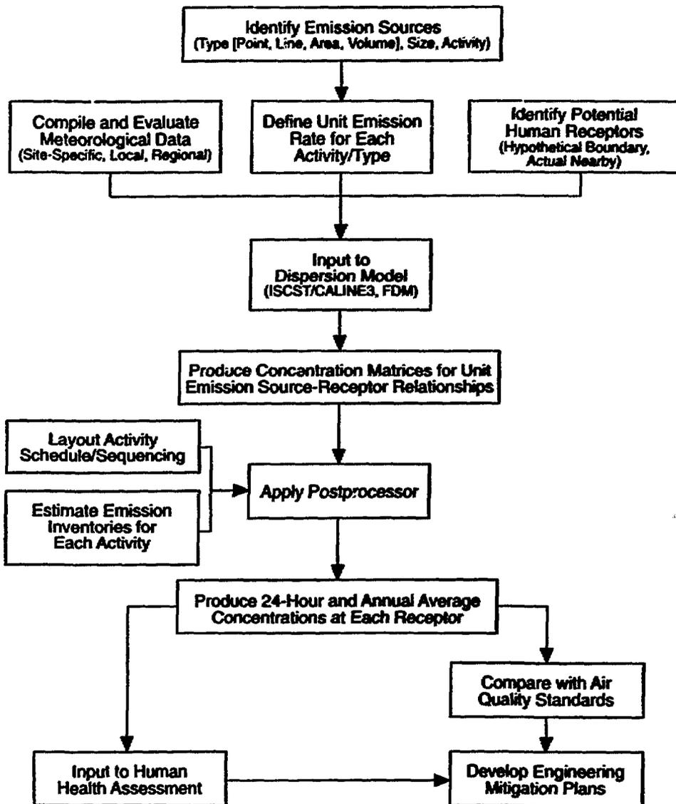
Fig. 3 Schematic Diagram of the General Process for Site-Specific Air Quality Modeling
