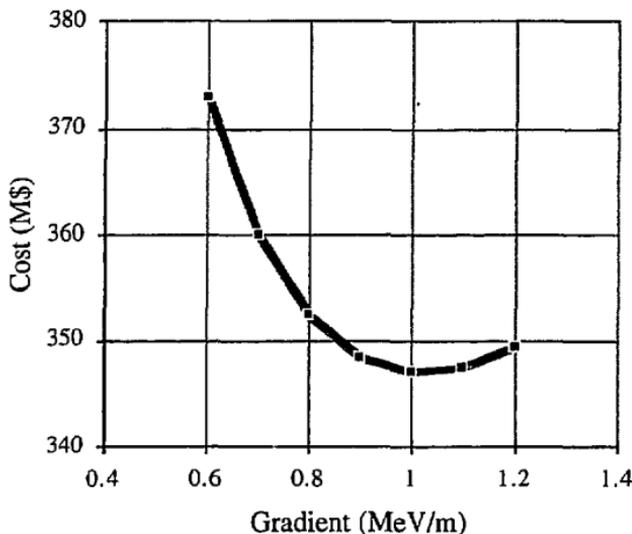
Figure 6. Cost v. accelerating field for a 1 GeV induction linac with  $I_{\text{beam}} = 1$  kA and  $T_p = 100$  ns. This estimate includes costs of 10 k\$/m for the accelerator building and 33 % for engineering, design and inspection.
