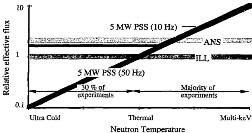
Fig. 2 Comparison of scientific effectiveness of existing ILL reactor (Grenoble) with proposed advanced neutron sources
