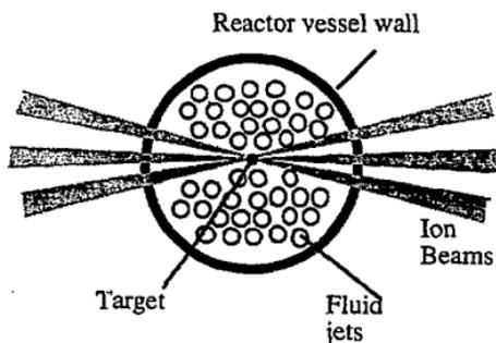
Fig. 1 Schematic representation of protection of a reactor wall with liquid jets
