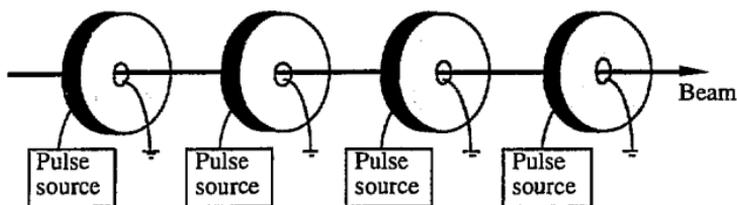
Figure 3. Schematic of an induction linac
