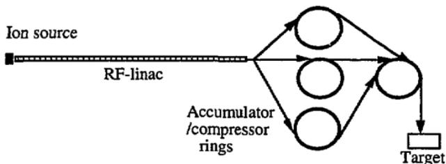
Figure 5. Pulse compression in an rf-accelerator system
