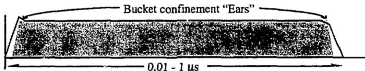
Figure 4 b. Induction linac voltage and current waveforms in non-resonant structure
