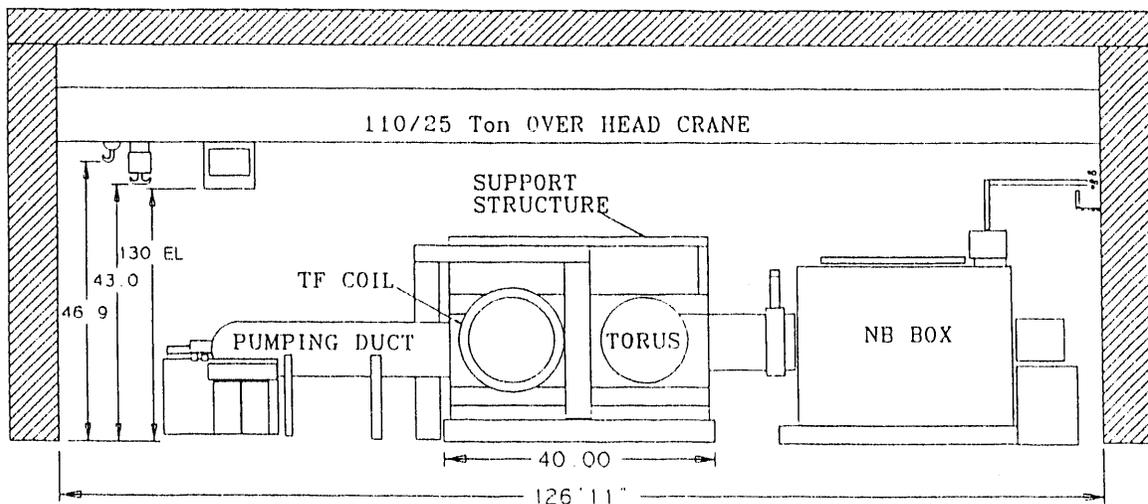
Fig. 2 TFTR Facility Elevation View.
