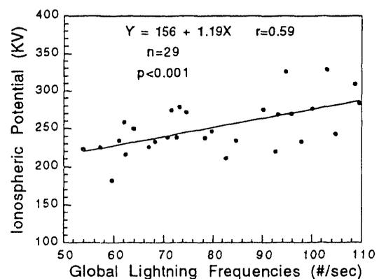
Figure 4. Relationship between 29 independently observed values of  $V_i$  and the corresponding globally integrated lightning frequency index.
