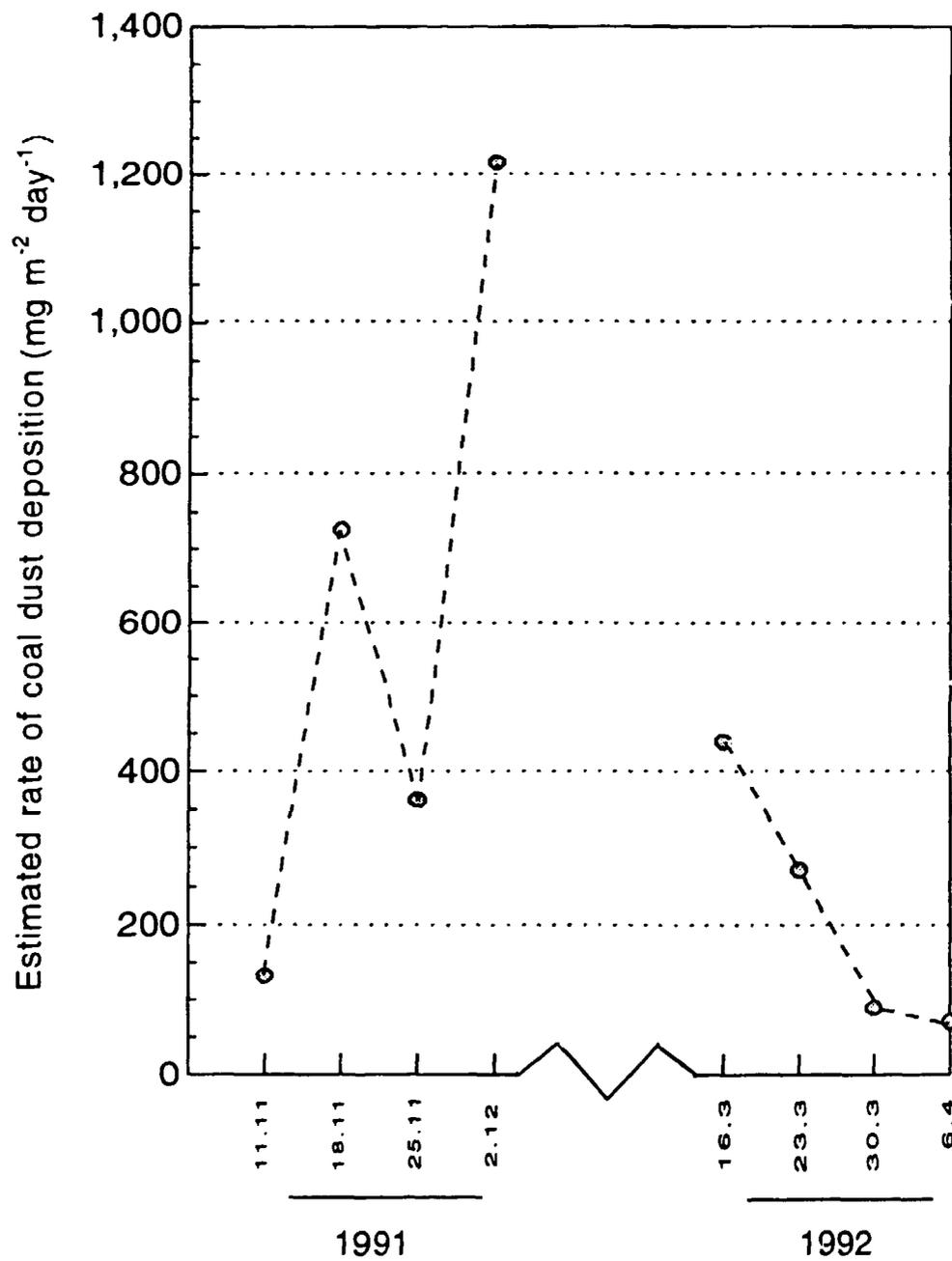
FIGURE 2 Variation in estimated coal dust deposition rate over the two four-weekly monitoring periods.
