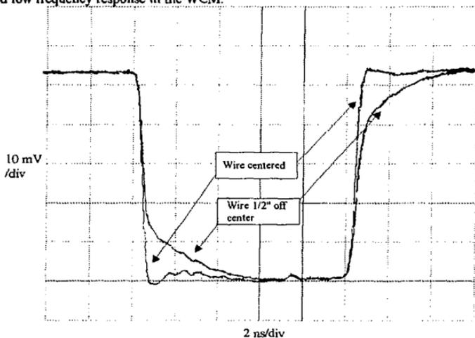
Fig. 5. WCM pulse response with centered and off-centered wire.
