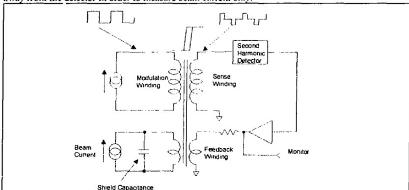
Figure 12. Simplified diagram of a DCCT
