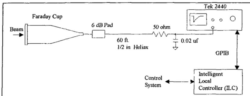
Fig. 10. Faraday cup beam charge measurement system.
