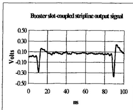
Figure 16. Measured frequency response of four tapered, slot-coupled striplines (left). Time response to beam bunches of single stripline (right) measured with an SCD5000 scan converter.
