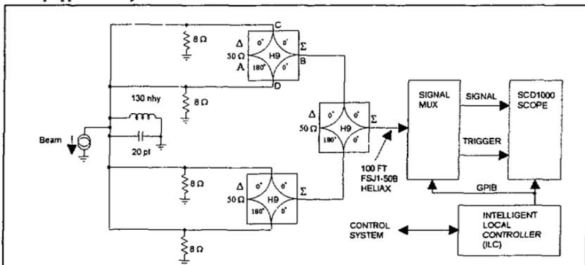
Fig. 3. Wall current monitor system connections.
