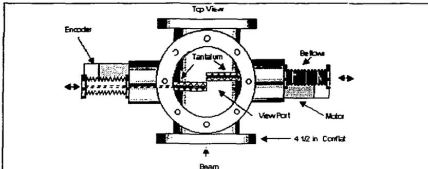
Figure 19. Drawing of single axis beam collimator.
