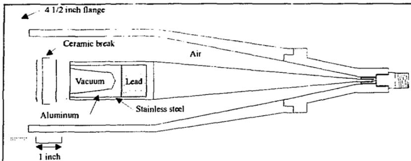
Fig. 9. 50 MeV Faraday cup. Connector is type N.
