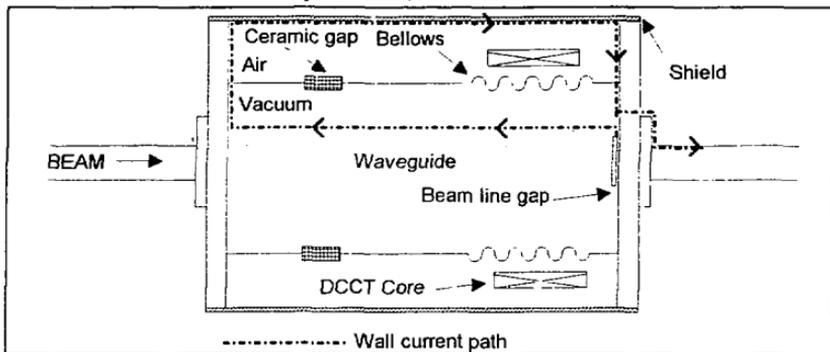
Figure 13. Simplified drawing of storage ring DCCT shield.
