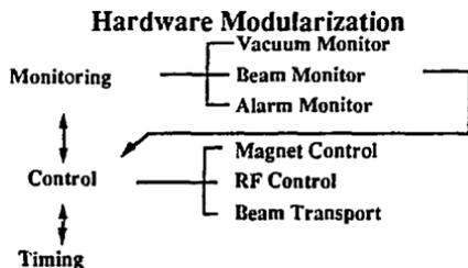
Fig.3 Separation of monitor path and control path
