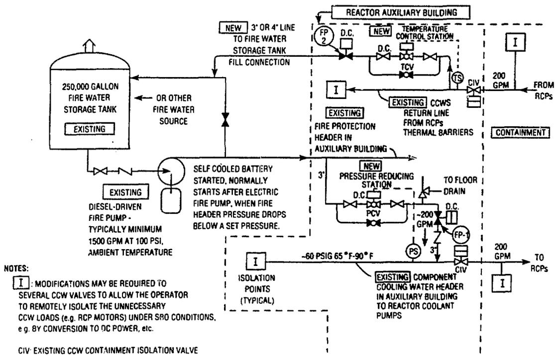
Figure 2. Example of independent seal cooling
