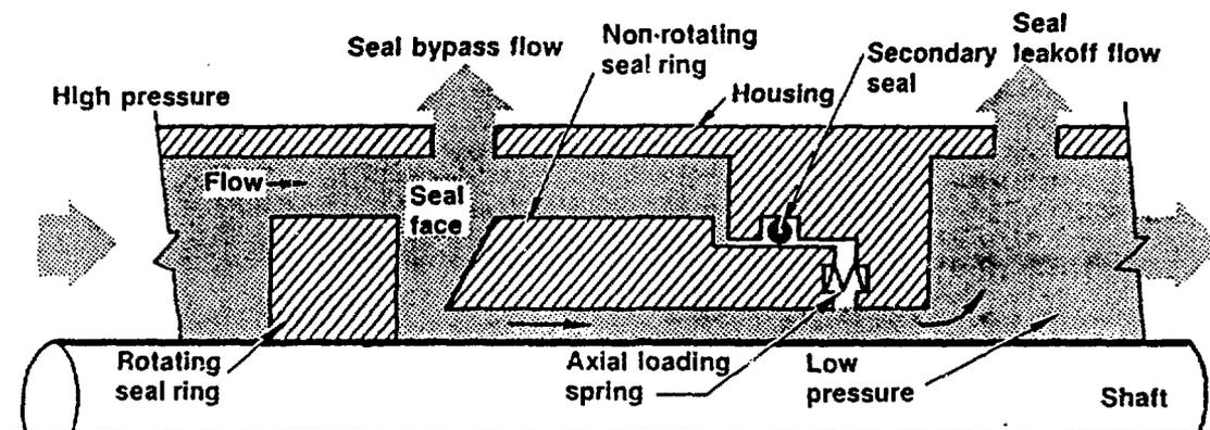
Figure 1. Simplified single stage of a RCP shaft seal
