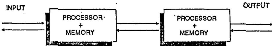
FIG.3 (b): A TWO PIPELINE TRANSPUTER SYSTEM
