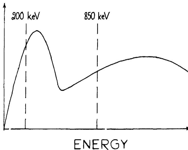
**Fig.8** Sum of the theoretical  $\beta$  spectra from Fig.3 with correction  $w(E)$  for the spectrometer resolution.
