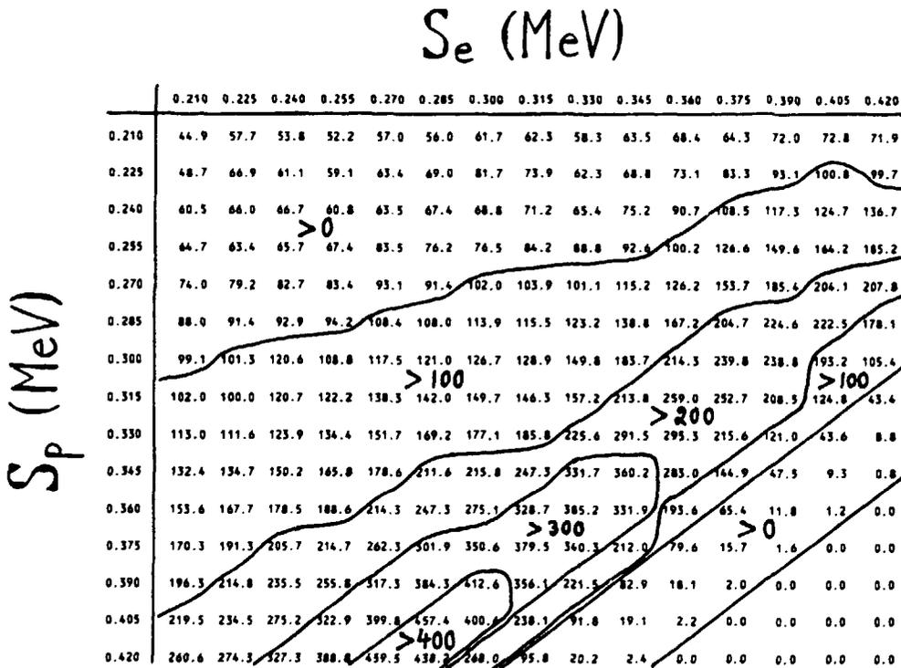
Fig.13 Simulated E0 matrix  $M_{E0}(S_e, S_p)$  for  $8 \cdot 10^7$  starting electron-positron pairs.
