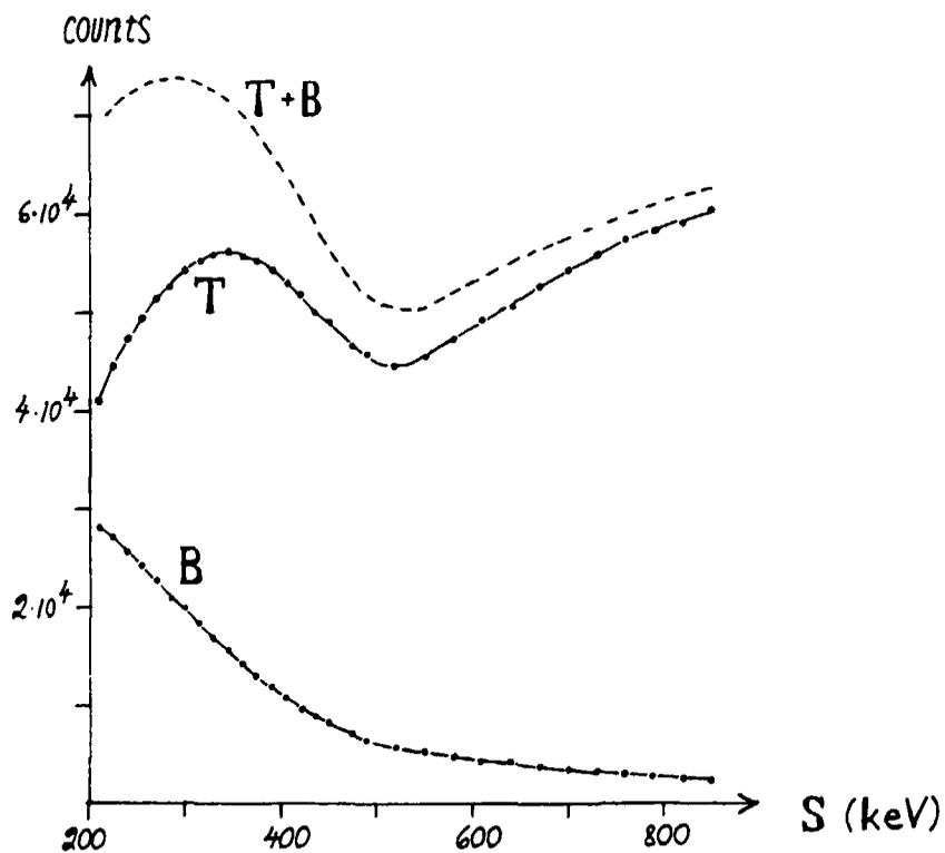
**Fig.7** Experimental singles electron spectra  $T(S)$  (transmission through the thorium foil) and  $B(S)$  (back-scattering from the foil), i.e. number of recorded electrons at different spectrometer settings  $S$ . Results are shown as dots, joined, for convenience, by curves. The experimental sum spectrum  $T + B$  is also indicated (dashed).
