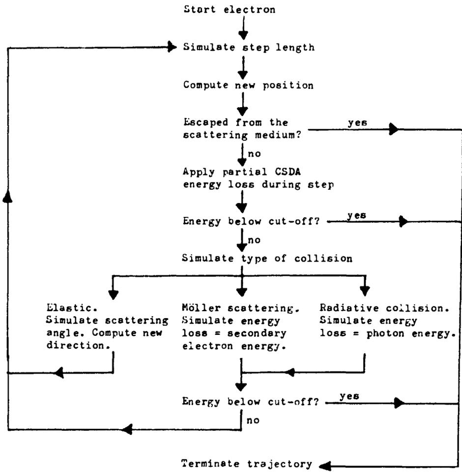
Fig.18 Principal flow diagram of RELECN, i.e. the basic principle of a typical scattering and energy loss subroutine (e.g. ELSIM1).
