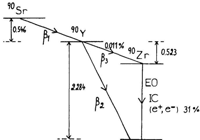
**Fig.2** Decay scheme. Energies are in MeV.
