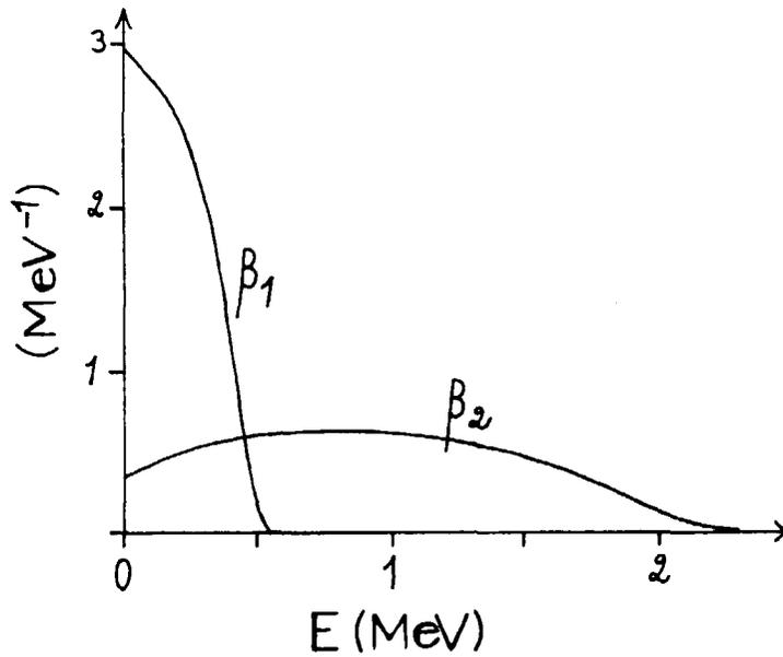
**Fig.3** The  $\beta_1$  and  $\beta_2$  energy distributions (number of electrons per unit energy), each normalized to unit area.
