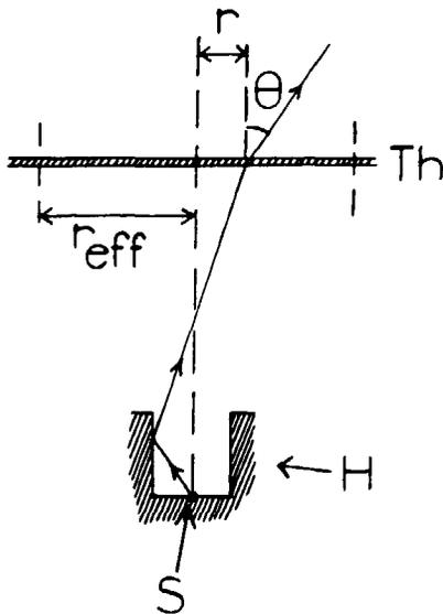
Fig.10 Scattering geometry of source holder and foil. An example of a possible scattering sequence is shown. The distance  $r$  from the foil hit point to the foil center is indicated. Notations otherwise as in Fig.1.
