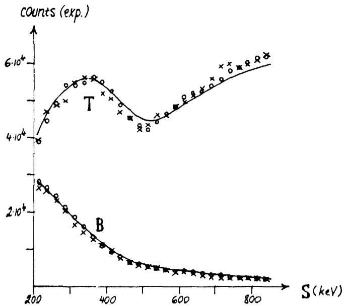
Fig.11d Simulated singles spectra compared with experimental, for the case  $r_{eff} = 5$  mm. Circles show simulated results for the angular interval of acceptance  $10^\circ < \theta < 50^\circ$ , while crosses show simulated results for  $25^\circ < \theta < 35^\circ$ . In both cases,  $f = 0.68$ . Full curves are experimental data from Fig.7. The number of starting simulated electrons was  $4 \cdot 10^6$  in each case.
