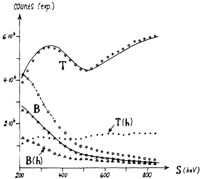
Fig.11c. Simulated singles spectra compared with experimental, for the case  $r_{eff} = 10$  mm. Symbols are as in Fig.11a, and  $f = 0.62$ . The number of starting simulated electrons was  $5 \cdot 10^6$ .
