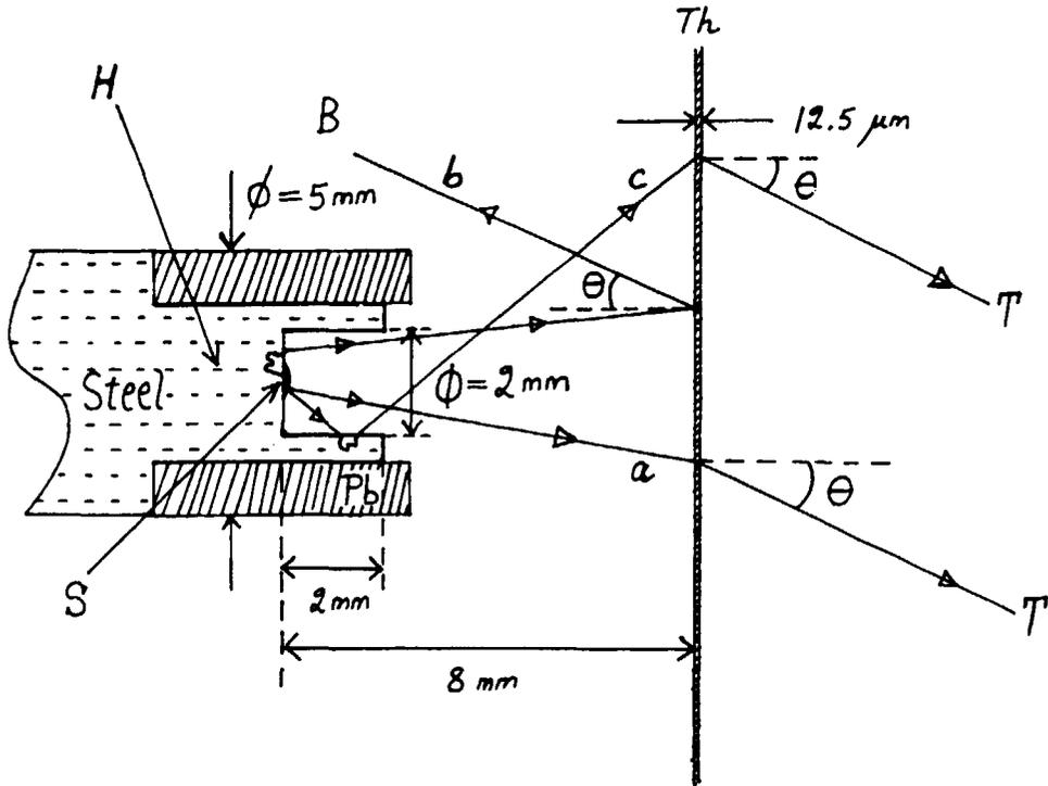
**Fig.1** Experimental geometry. S = source, H = source holder (cylindrical), Th = thorium foil, B = backscattered lepton, T = transmitted lepton,  $\theta$  = acceptance angle. A few electron (or positron) trajectories are schematically indicated. Trajectory (a): direct hit of foil and transmission; trajectory (b): backscattering from bottom of cavity, foil hit, and backscattering; trajectory (c): scattering from cavity wall, foil hit, and transmission.
