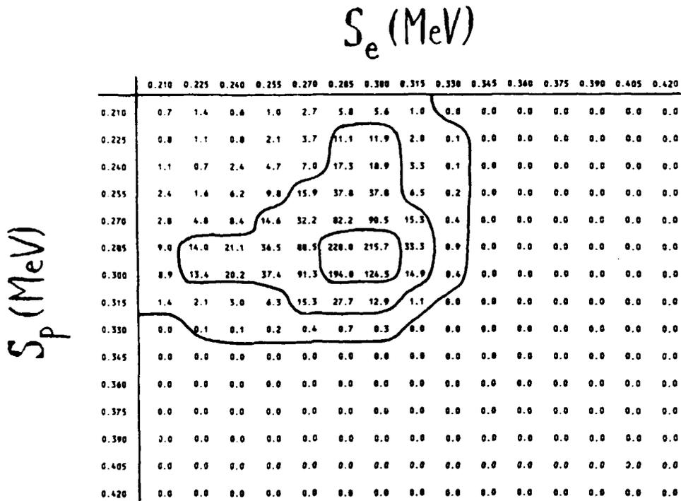
**Fig.17** Example of a simulated electron-positron coincidence matrix  $M_H(S_e, S_p)$  due to hypothetical events. In the case shown, the initial energies of the electron and the positron are both 300 keV.
