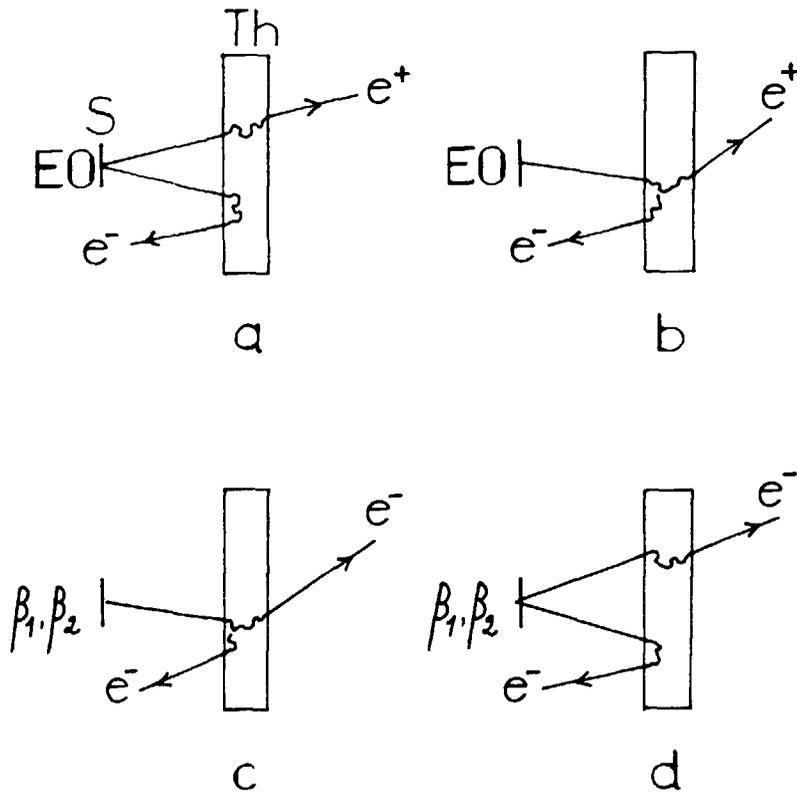
**Fig.5** Schematic illustration of different scattering processes in the thorium foil.
