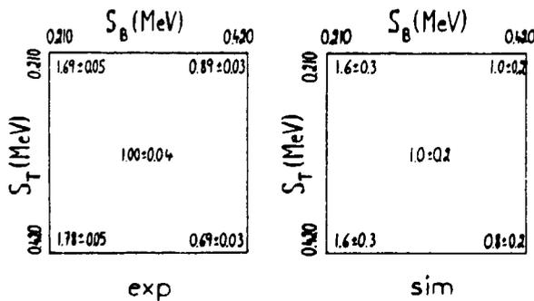
Fig.16 a) Simulated Møller coincidence matrix  $M_M(S_B, S_T)$ . b) Rescaled simulated and experimental Møller coincidence matrices. Values in the center and the corners are indicated with estimated statistical errors.
