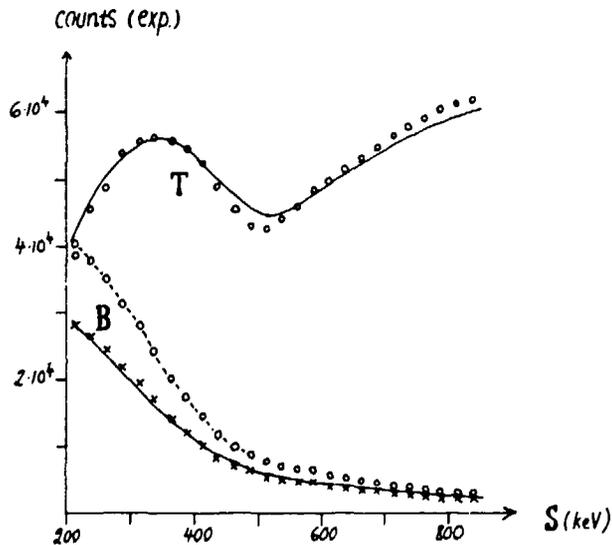
Fig.11b. Simulated singles spectra compared with experimental, for the case  $r_{eff} = 4$  mm. Symbols are as in Fig.11a, and  $f = 0.70$ . The number of starting simulated electrons was  $10^7$ .
