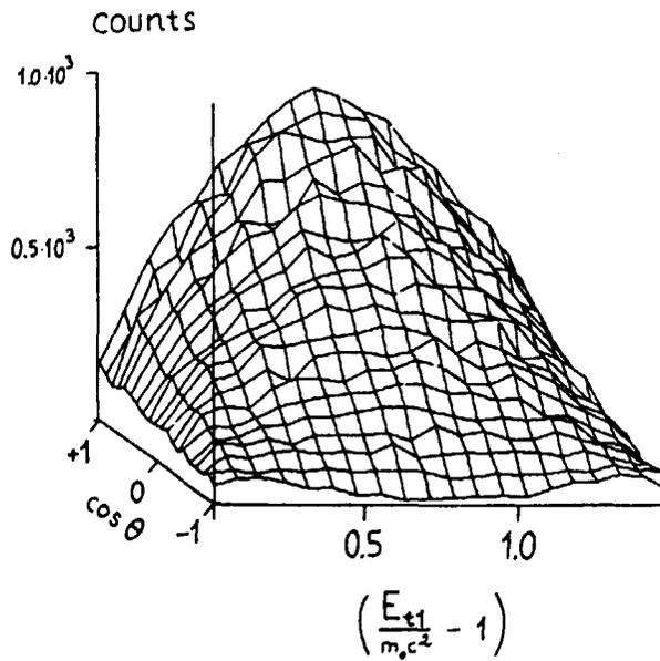
**Fig.4** Sampling test (using the rejection method) of the energy-direction distribution  $P_{E0}(E_{t1}, \cos \theta)$  of the electron and positron pair created in the  $E0$  decay.  $E_{t1}$  is the energy of one lepton,  $\theta$  is the angle between the directions of motions.
